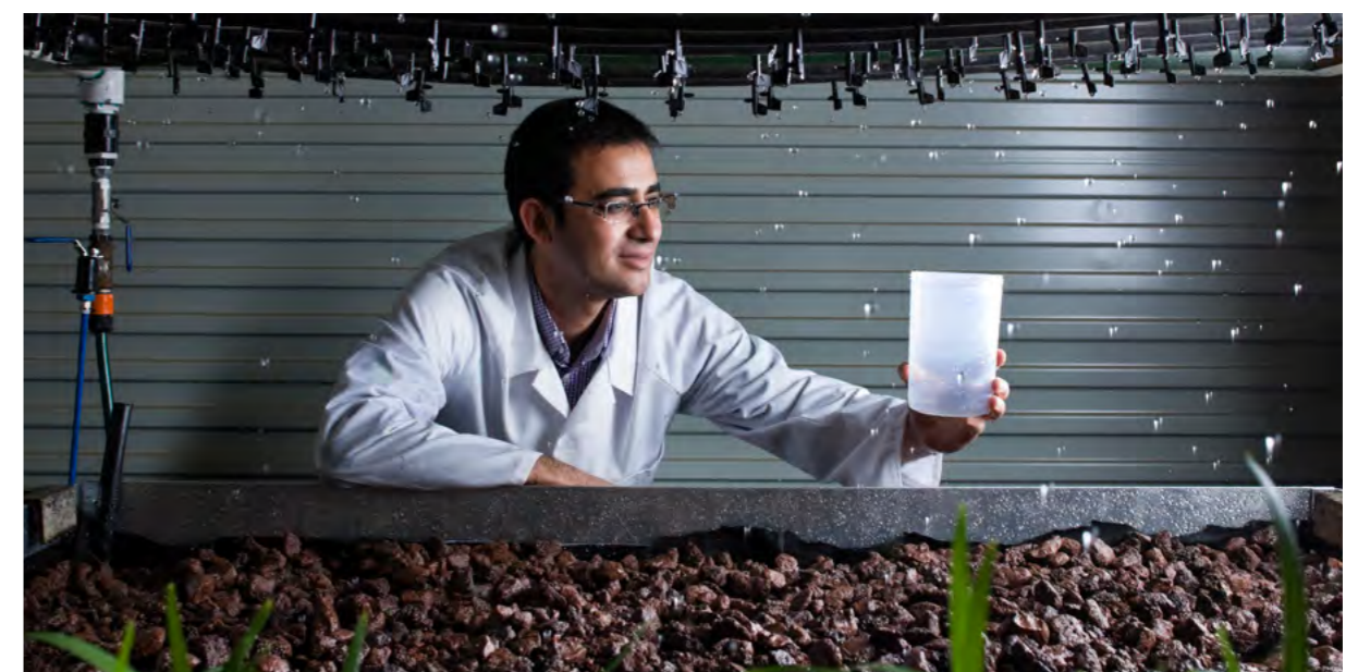
PhD Student Mostafa Razzaghmanesh working on the rainfall simulator at UniSA Mawson Lakes Campus. Photo courtesy of Sam Noonan, www.samnoonan.com.au
