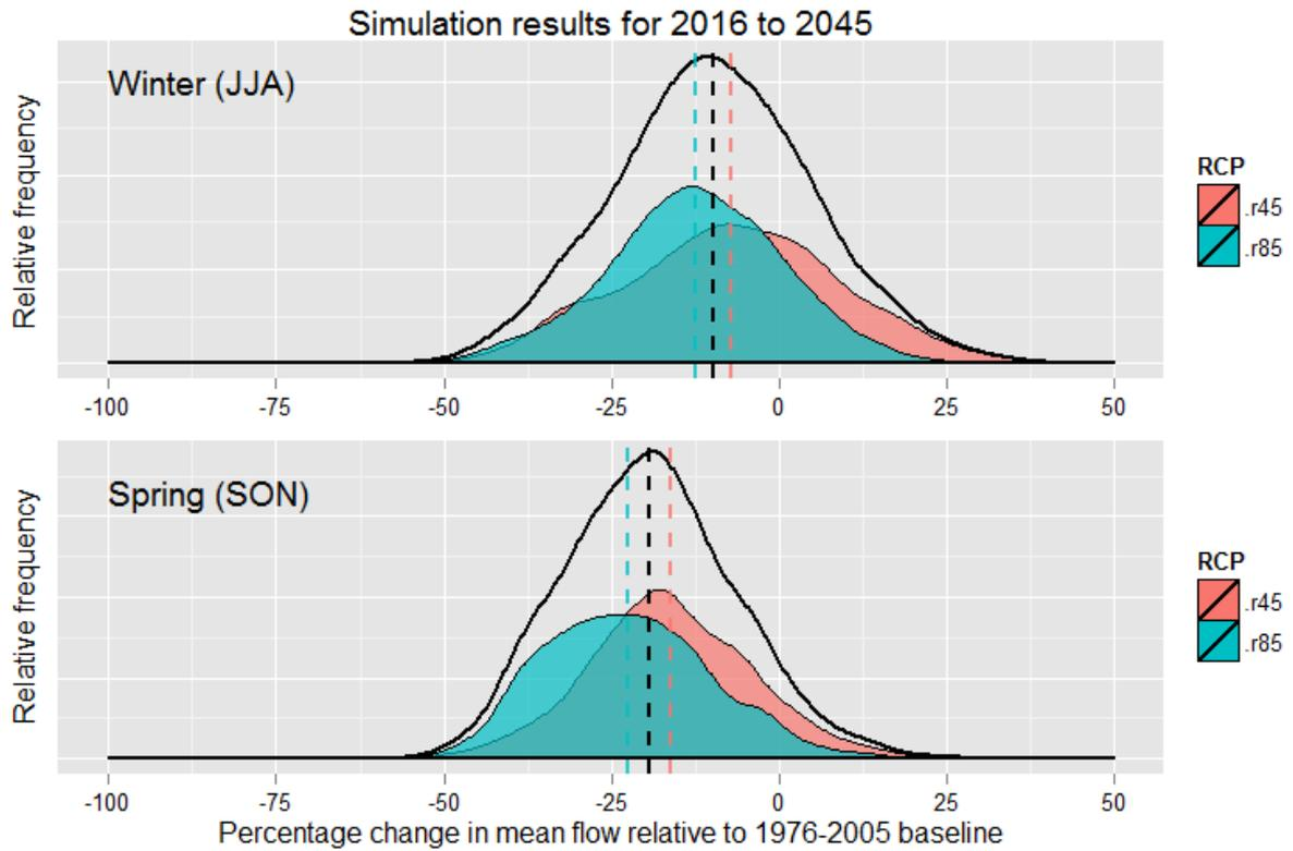
**Figure 6: Percentage change in mean winter and spring flow at Houlgrave Weir for 2016 to 2045 for all GCMs and hydrological models, presented for two RCPs.**
