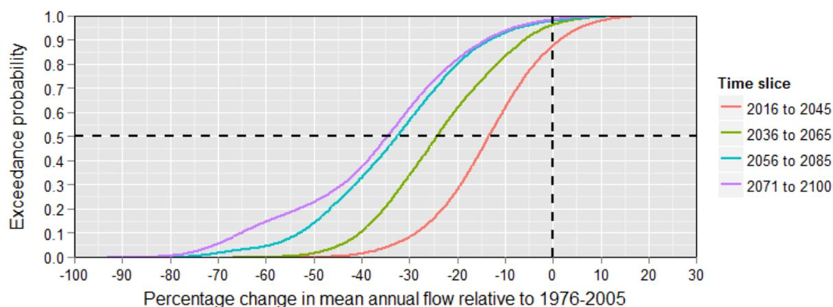
**Figure 2: Cumulative distribution function of the projected change in mean annual flow relative to the 1976 to 2005 baseline, for four future time slices. The plot combines results from all 15 GCMs, 2 RCPs, 4 hydrological models and 100 NHMM simulations.**
