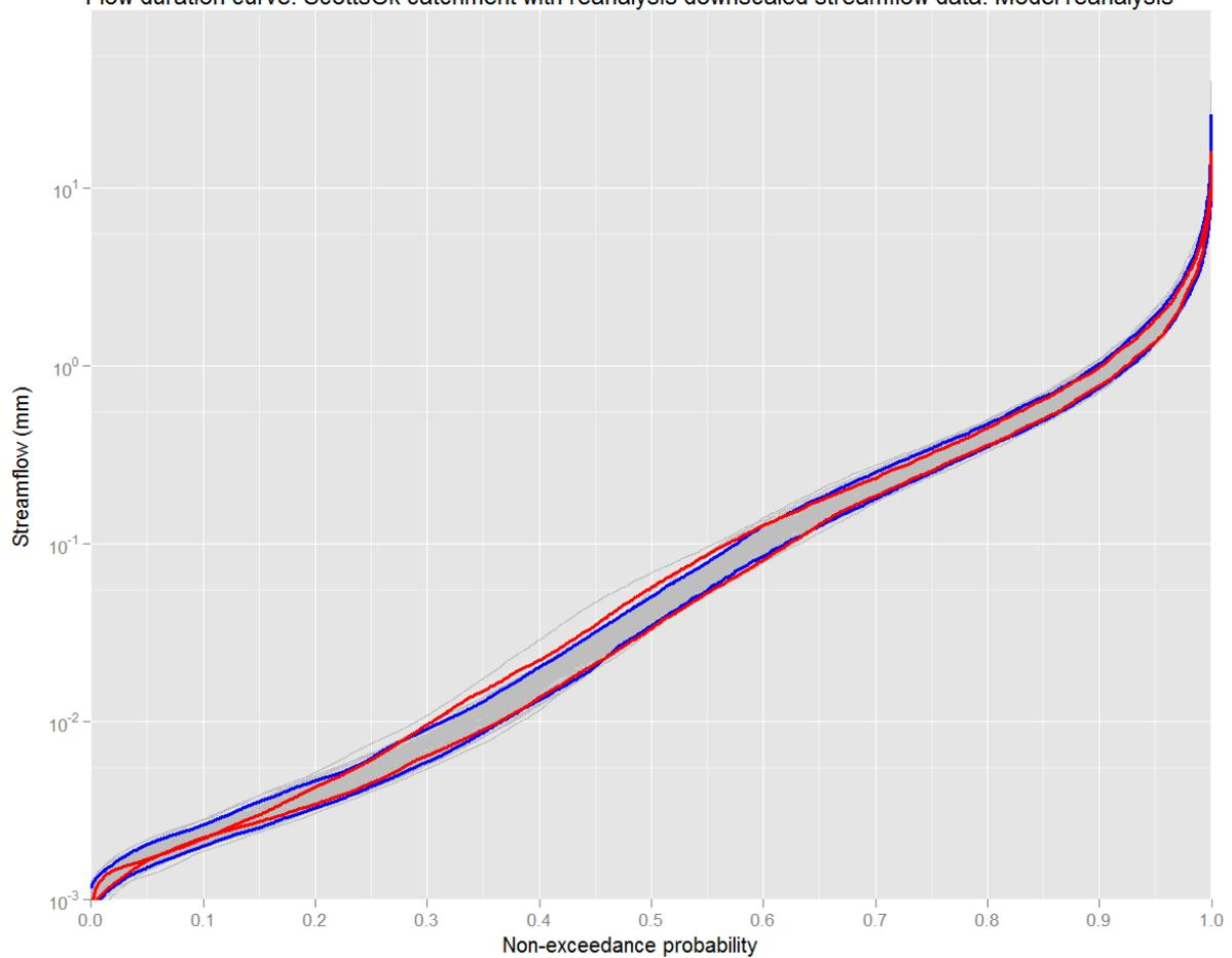
**Figure 32: Grey lines are the 100 simulations. Blue lines are the 5<sup>th</sup> and 96<sup>th</sup> value calculated at each exceedance probability (i.e. doesn't represent a single flow duration curve). Red lines are the flow duration curves one would get if using the runs obtained from the 5<sup>th</sup> and 96<sup>th</sup> ranked simulations by annual average rainfall.**
