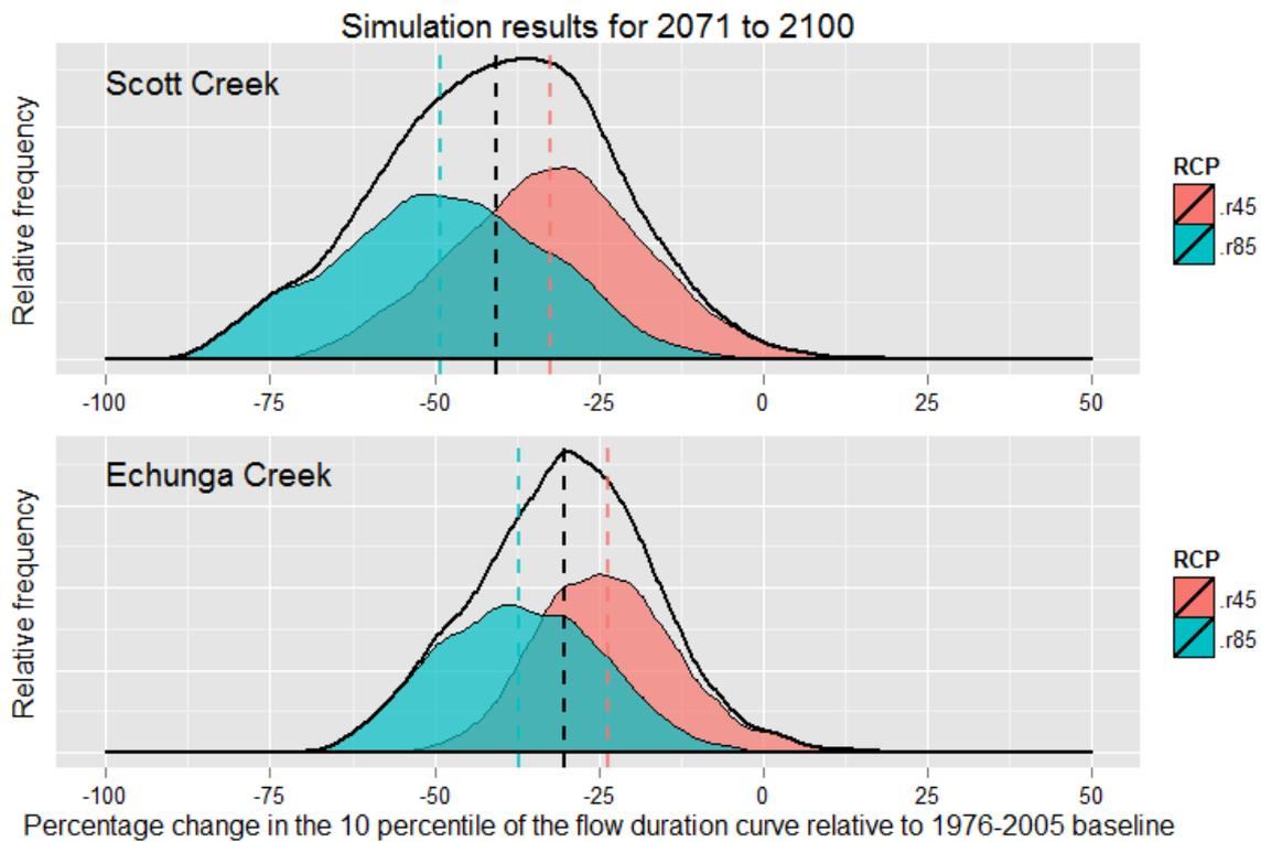
**Figure 18: Percentage change in the 10th percentile of the daily flow duration curve for the 2071 to 2100 time slice at Scott Creek (upper panel) and Echunga Creek (lower panel), for all GCMs and hydrological models.**
