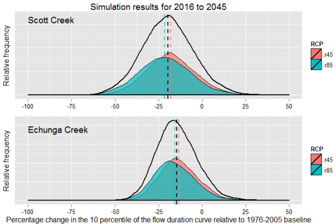
**Figure 17: Percentage change in the 10th percentile of the daily flow duration curve for the 2016 to 2045 time slice at Scott Creek (upper panel) and Echunga Creek (lower panel), for all GCMs and hydrological models.**
