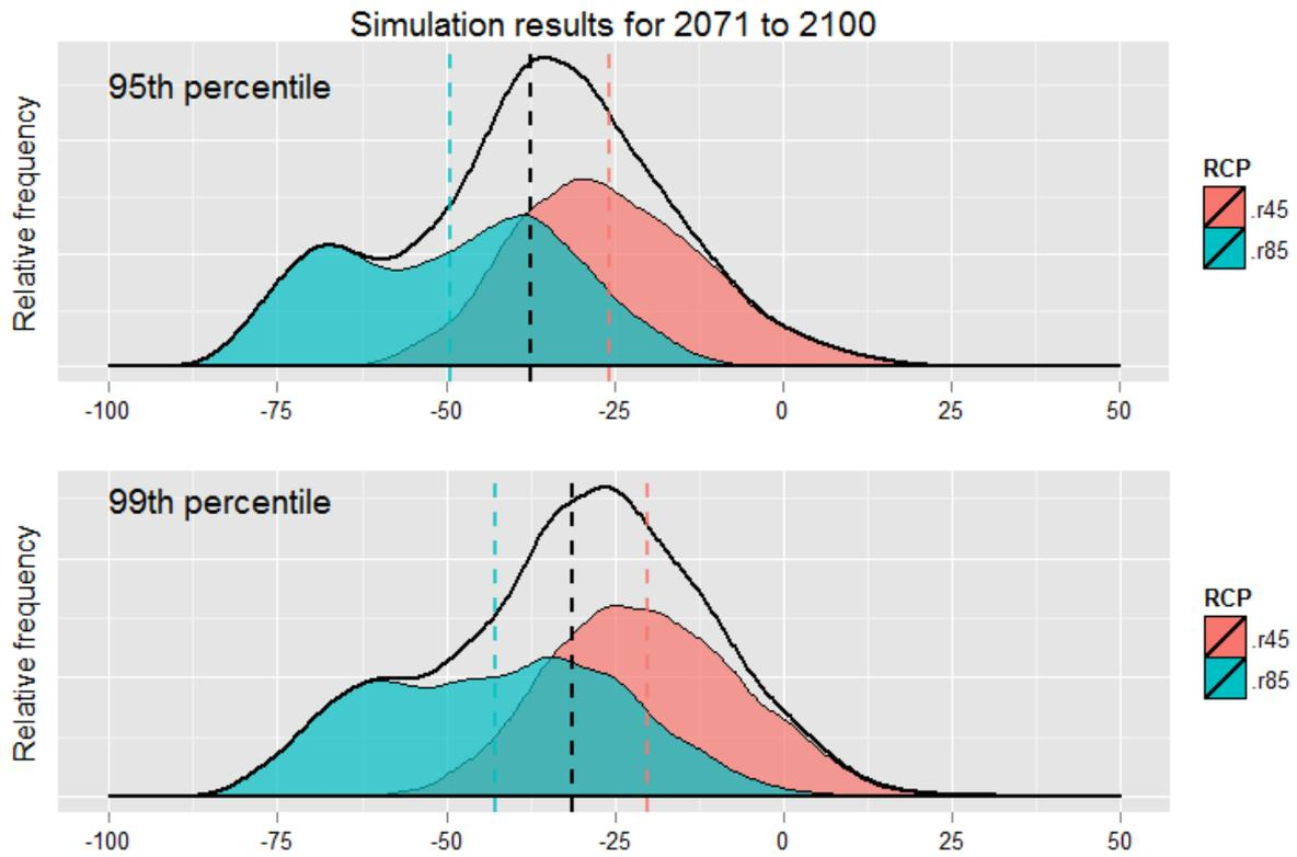
**Figure 20: Percentage change in the 95<sup>th</sup> and 99<sup>th</sup> percentile daily flow at Houlgrave Weir for all GCMs and hydrological models for 2016 to 2045 and 2071 to 2100**
