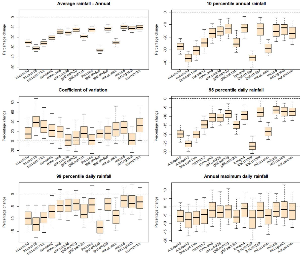
**Figure 27: Box and whisker plot presented by GCM at Houlgrave Weir for the 2071 to 2100 time slice based on RCP 8.5, using hydrological model  $g_{1.1}$ , at the annual time scale. Similar plots can be generated for each time slice, RCP, hydrological model and season.**
