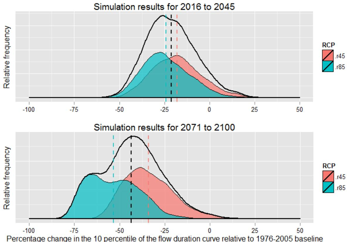
**Figure 16: Percentage change in the 10th percentile of the daily flow duration curve calculated for spring at Houlgrave Weir for all GCMs and hydrological models, for the 2016 to 2045 and 2071 to 2100 time slices**
