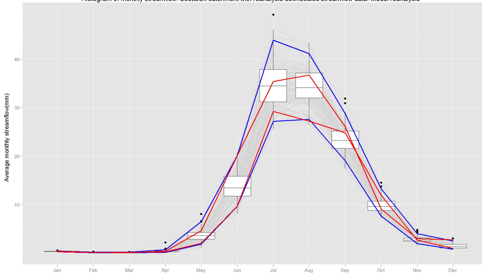
**Figure 34: Monthly average streamflow from the 100 reanalysis simulations. Blue lines are the 5<sup>th</sup> and 96<sup>th</sup> ranked values calculated separately for each month. Red lines are the monthly flows from the 5<sup>th</sup> and 96<sup>th</sup> ranked simulations calculated based on annual average rainfall.**
