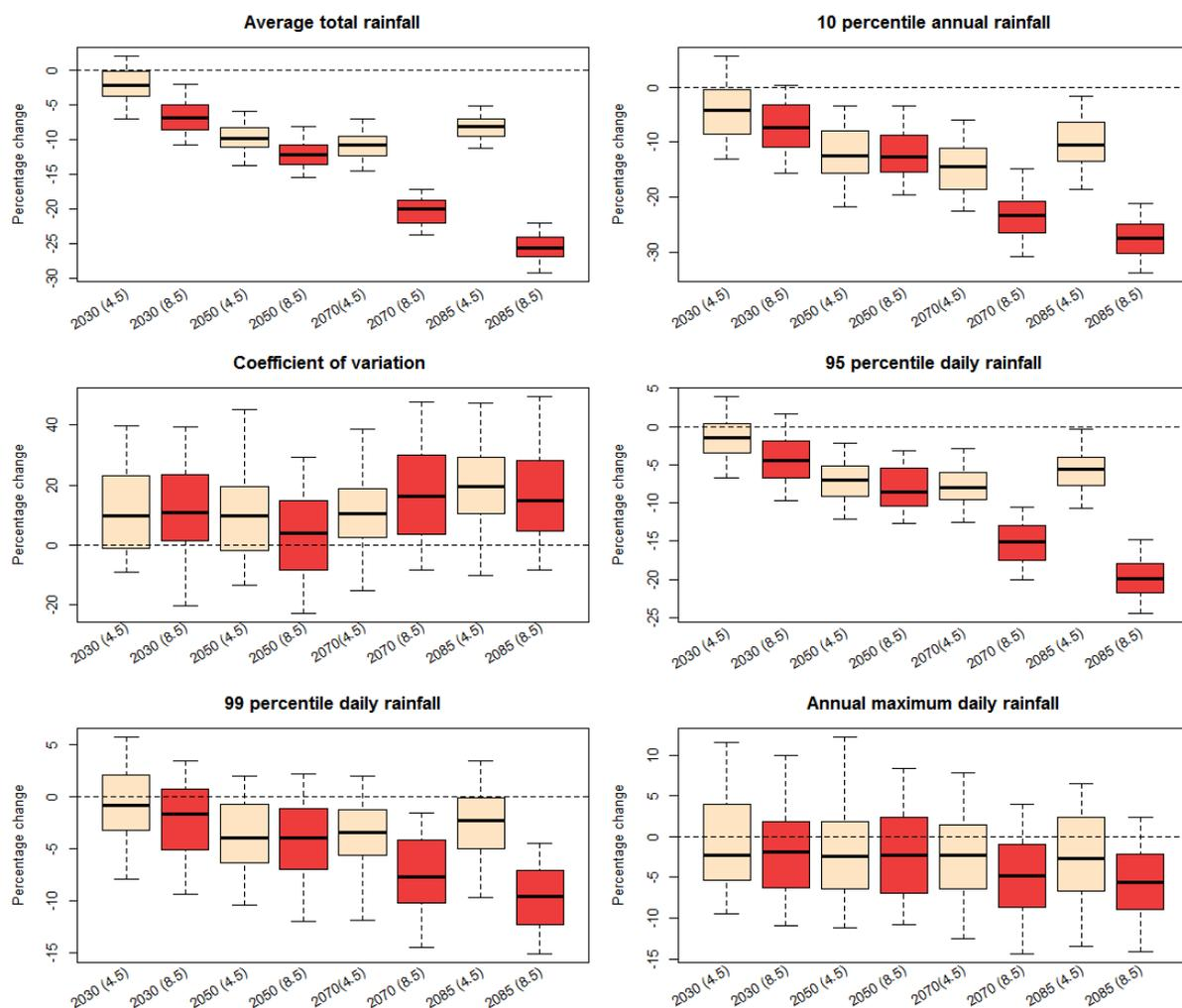
**Figure 26: Box and whisker plot presented by time slice at Houlgrave Weir for the ACCESS 1.0 GCM, hydrological model  $g_{1.1}$ , at the annual time scale. Similar plots can be generated for each GCM, hydrological model and season.**
