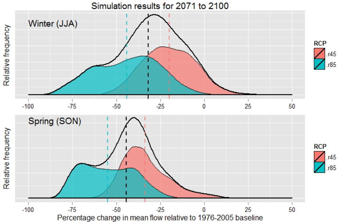
**Figure 7: Percentage change in mean winter and spring flow at Houlgrave Weir for 2071 to 2100 for all GCMs and hydrological models, presented for two RCPs.**
