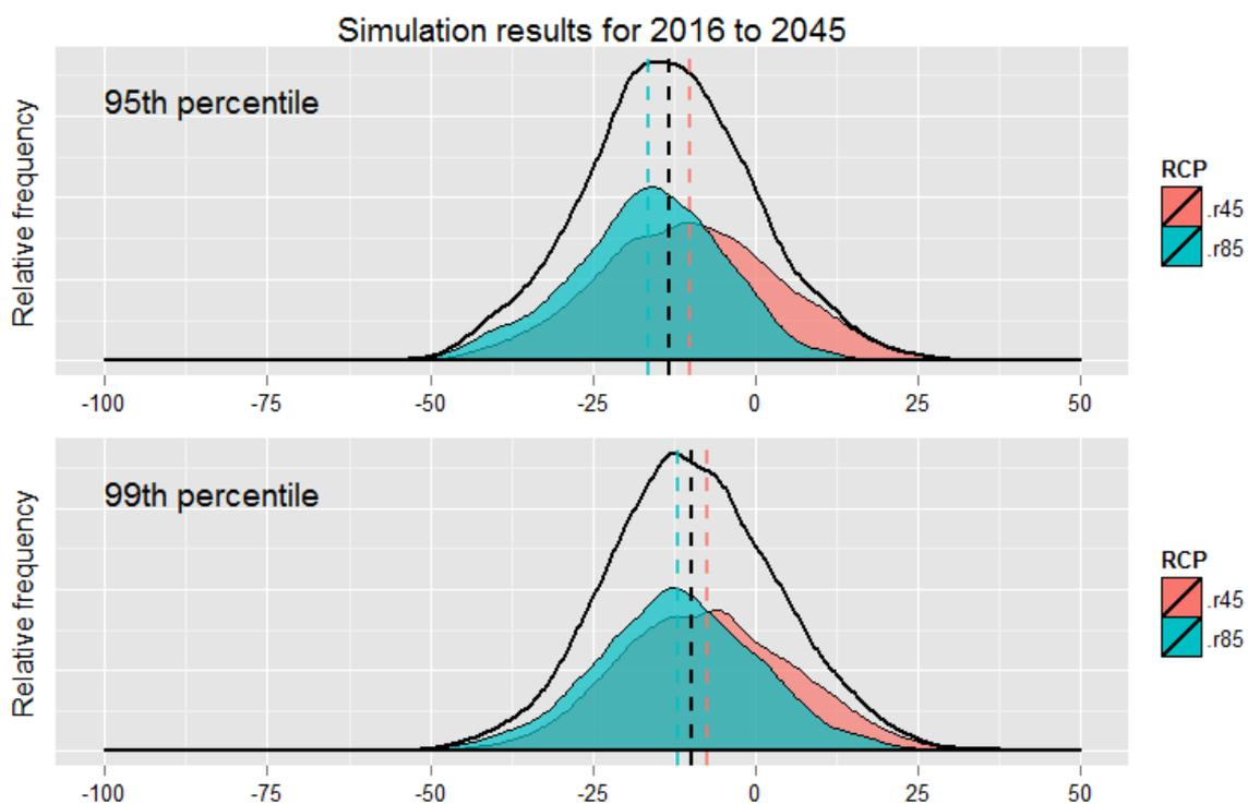
**Figure 19: Percentage change in the 95<sup>th</sup> and 99<sup>th</sup> percentile daily flow at Houlgrave Weir for all GCMs and hydrological models for 2016 to 2045 and 2071 to 2100.**
