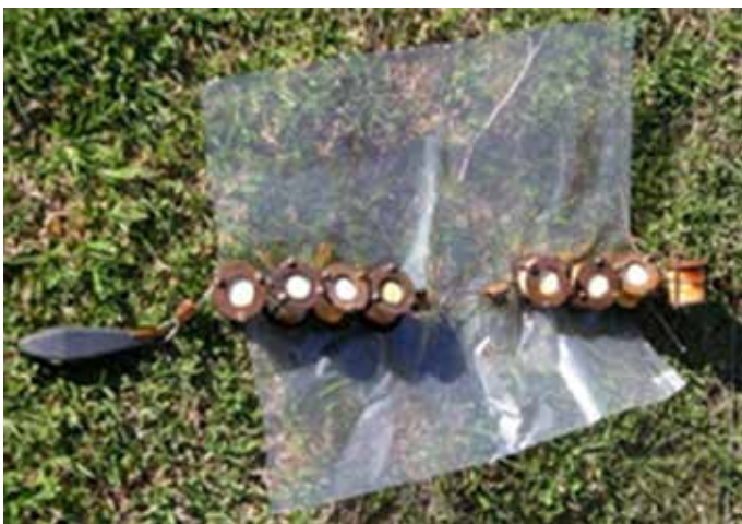
Figure A16.1 Diffusion chambers used in the pathogen decay study.
