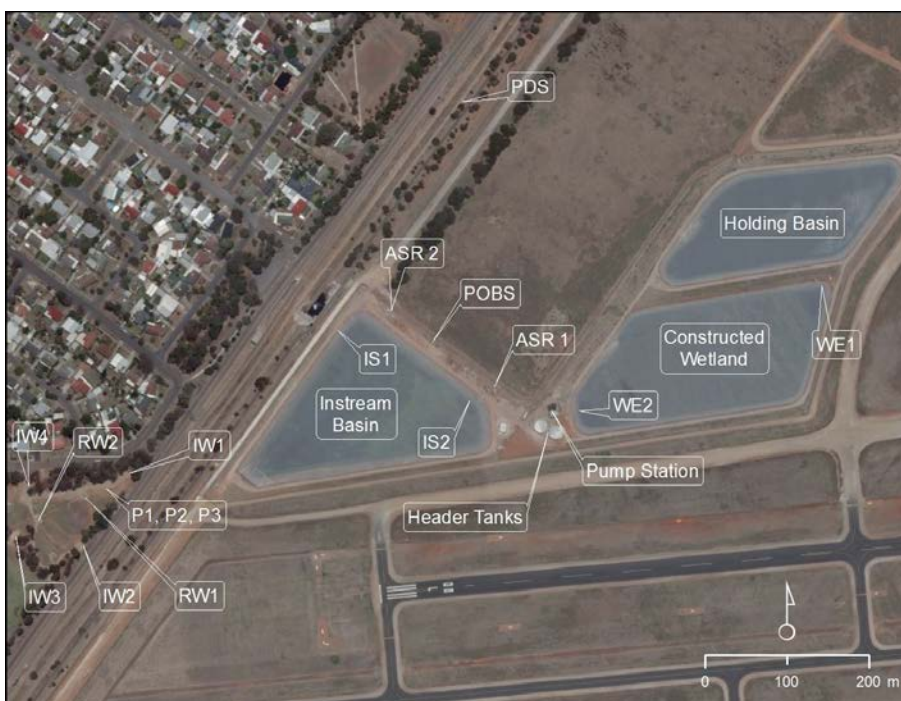
Figure 8 Parafield stormwater harvesting system layout showing scheme sampling points.
