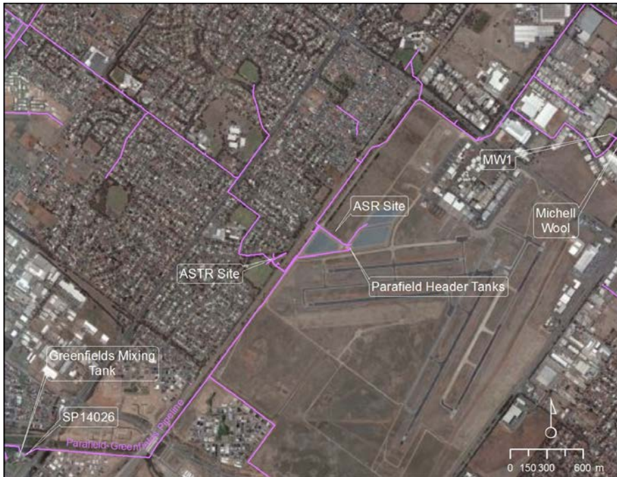
Figure 7 Parafield recycled stormwater distribution pipeline (purple line), sampling points at inlet to Greenfields Mixing Tank (SP14026) and Mitchell Wool (MW1). Parafield-Greenfields Pipeline is a dedicated pipeline from the Parafield header tanks to the Greenfields Mixing Tank.
