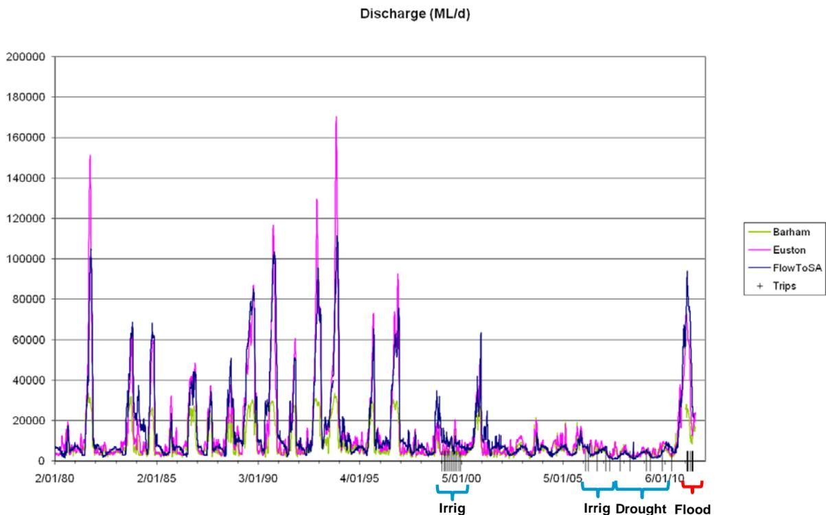
Figure 5. Murray River hydrographs at three gauging stations from 1980-2011 showing discharge prior to and during periods when river metabolism measurements were made. Sampling trips are indicated by vertical lines crossing the x-axis. The sampling times are categorized into periods of irrigation flows (Irrig), drought flows (Drought) and flood flows (Flood) as described in the text.
