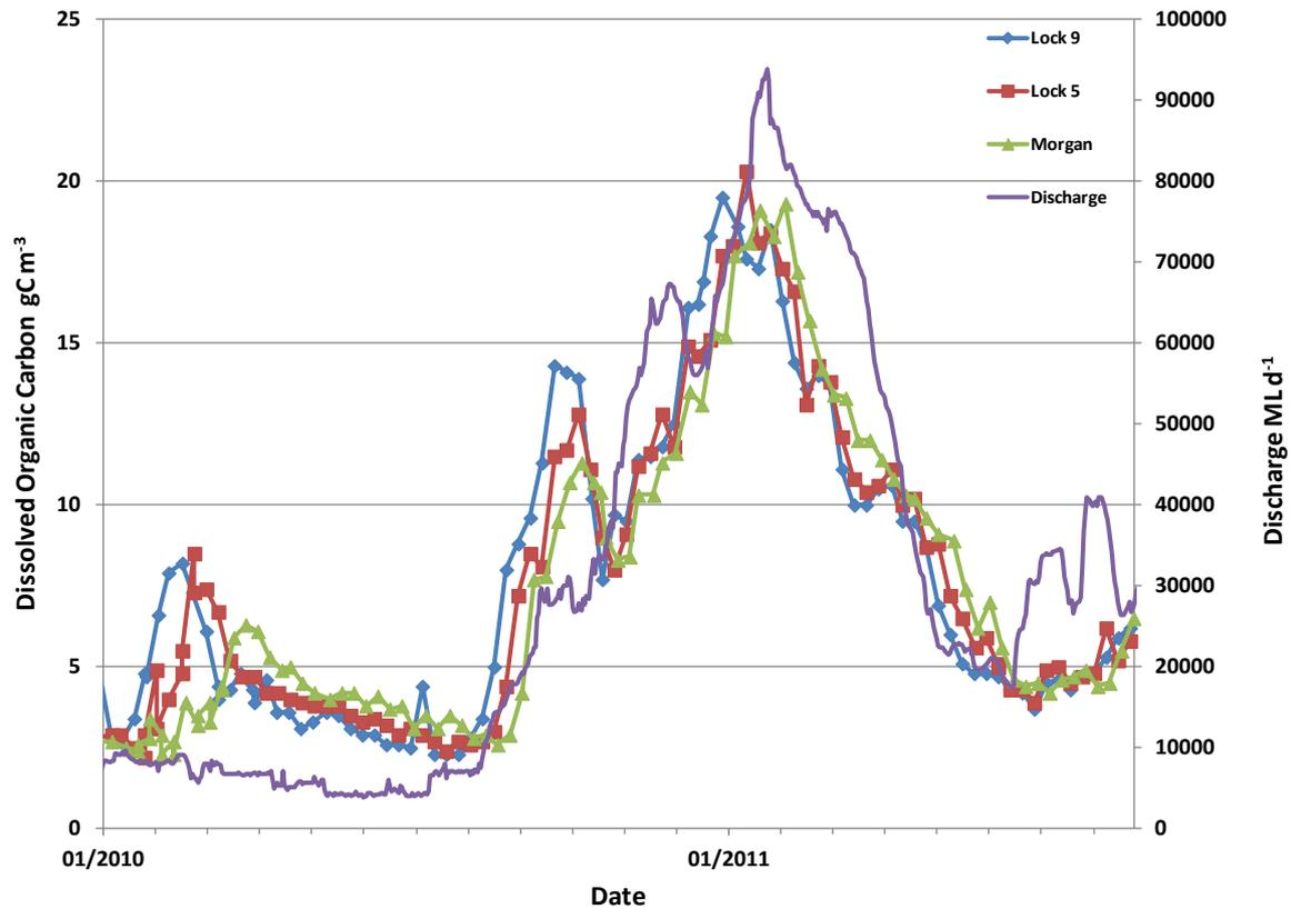
Figure 14. Time series of dissolved organic carbon concentrations and river discharge at Lock 9, Lock 5 and Morgan prior to and during the 2010-2011 flood peak. Data provided from the MDBA monitoring program.
