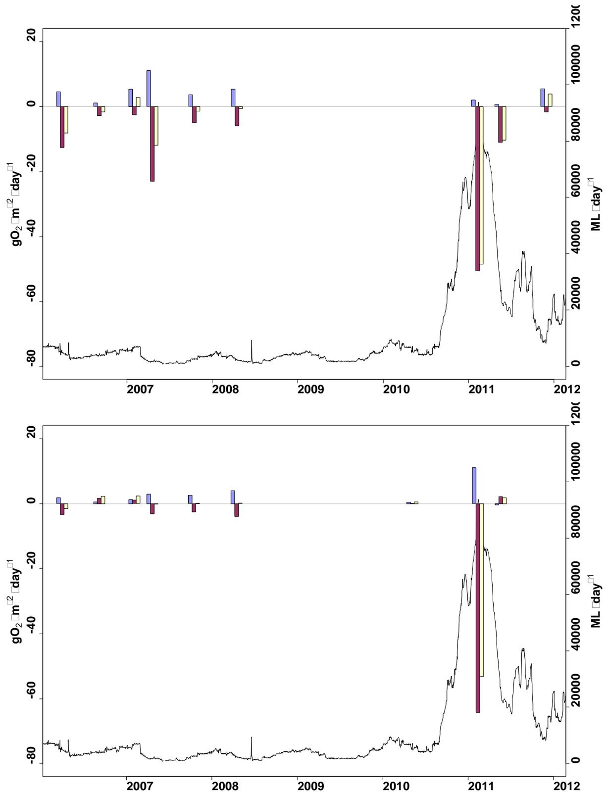
Figure 12. Non-planktonic rates of *GP* (blue bars), *CR* (red bars) and *NP* (yellow bars) measured in the weir pool upstream of Lock 4 (top) and in the river downstream of Lock 5 (bottom) in South Australia before, during and after the flood flows shown by the discharge hydrograph.
