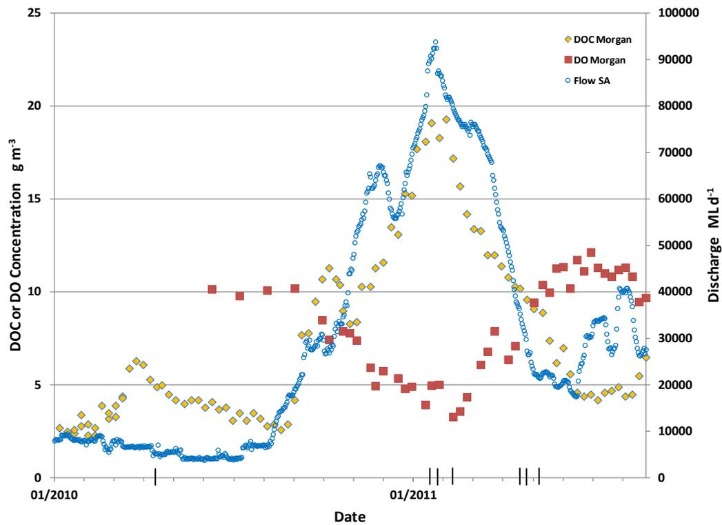
Figure 13. Changes over time in the discharge to SA and the concentrations of dissolved oxygen and dissolved organic carbon measured in the Murray River at Morgan in South Australia. Vertical lines on x-axis indicate times of metabolism measurements.
