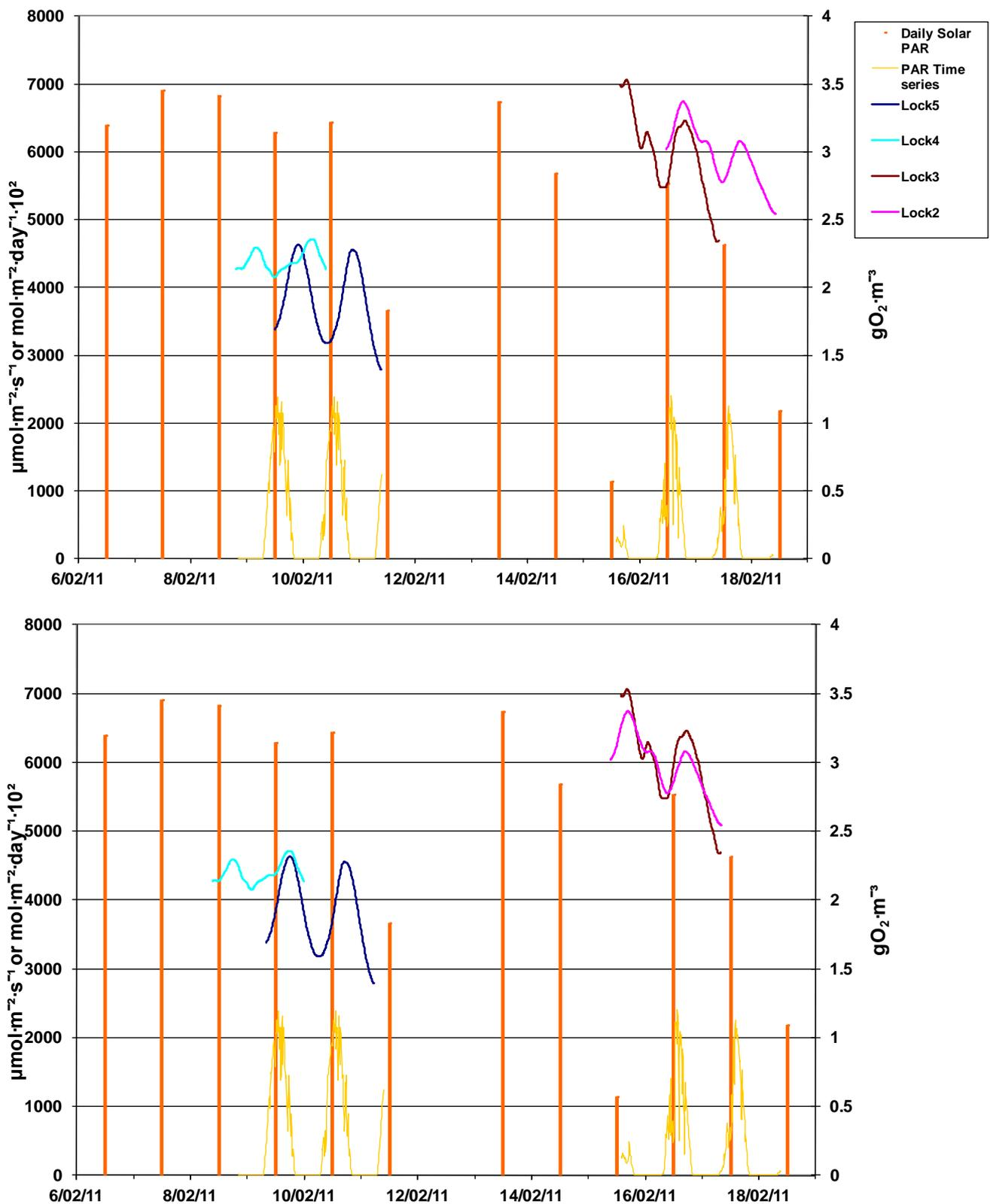
Figure 16. Daily solar photosynthetically active radiation (PAR) and the time series of PAR and oxygen concentrations during metabolism measurements at Lock 5, 4, 3, and 2. Upper graph shows oxygen curves as measured, lower graph shows oxygen curves shifted to align with prior light period. Daily PAR values multiplied by  $10^2$  to fit on axis scale.
