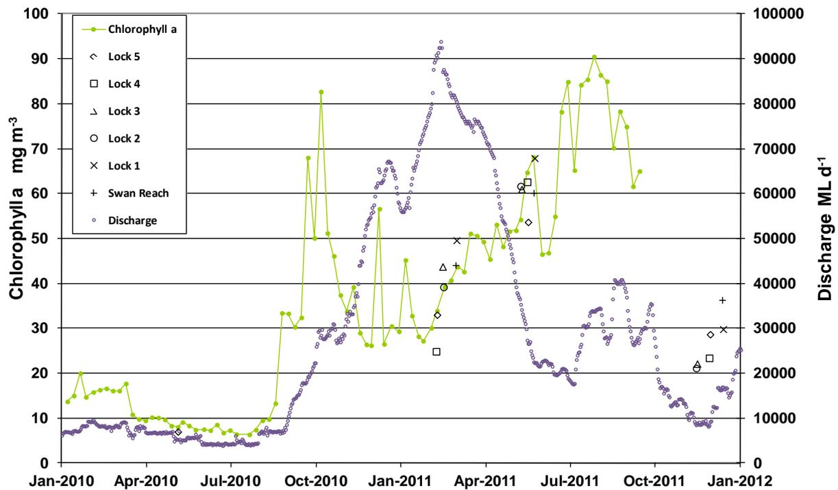
Figure 19. Chlorophyll a concentrations monitored at Morgan by the MDBA, and concentrations determined during metabolism measurements at sampling sites (symbols) compared with the river discharge to South Australia.
