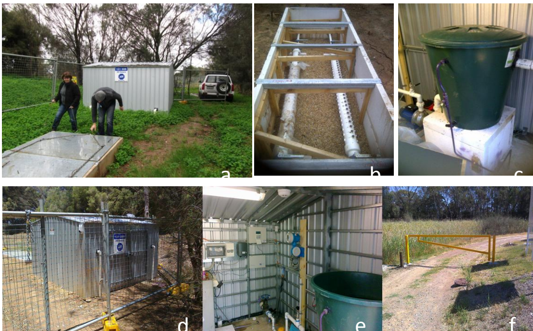
Figure 7 Photos of experimental rig: (a) Biorig pit and control room; (b) Biorig section showing coupon housing; (c) Rig header tank; (d) Secured (fenced and alarmed) pump shed and site; (e) Flow control instrumentation, (f) Manual boom gate to restrict site access.
