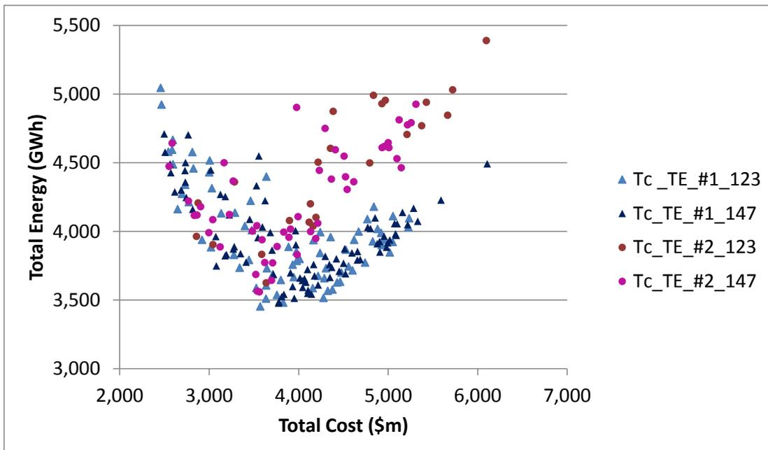
**Figure 47: Costs and energies of non-dominated solutions using 2 different seeds (0.123 and 0.147) for the 2013 scenario with Priority Sets #1 and #2, where Tc = total cost and TE = total energy**
