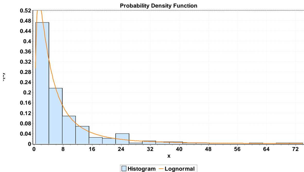
**Figure 36: Observed rainwater tank sizes from 277 households in Metropolitan Adelaide and fitting of the observed tank sizes to log-normal distribution (Kolmogorov-Smirnov test statistic = 0.077, accepted at 5% significant level; p-value = 0.0816)**
