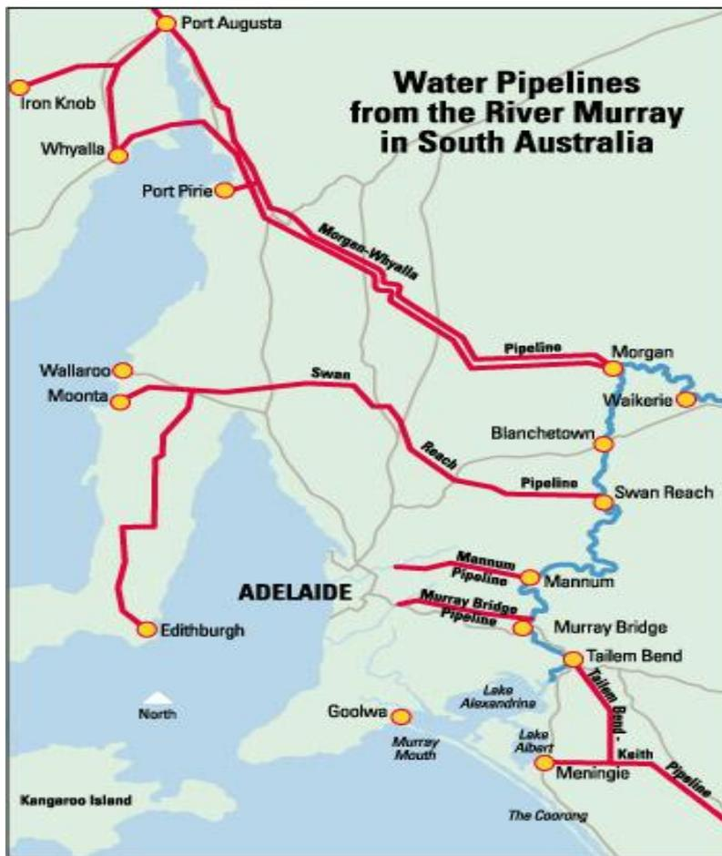
Figure 6: Pipelines to draw water from the River Murray in South Australia: water drawn from Murray Bridge, Mannum and Swan Reach is used to supply water to Metropolitan Adelaide (source: <http://www.murrayriver.com.au/about-the-murray/water-use-and-consumption/> )
