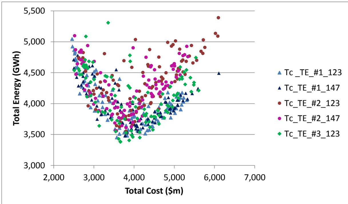
Figure 51: Total costs and total energy of the solutions found for the 2013 scenario with Priority Sets #1, #2 and #3, where Tc = total cost and TE = total energy
