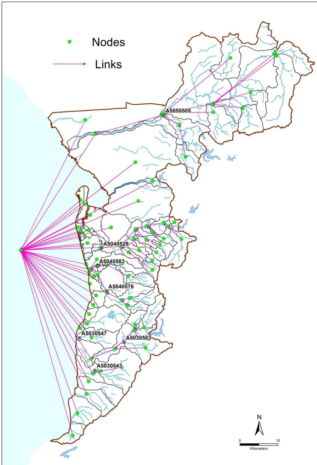
**Figure 31: Gauging stations used for calibration and the node-link network of the catchment model**
