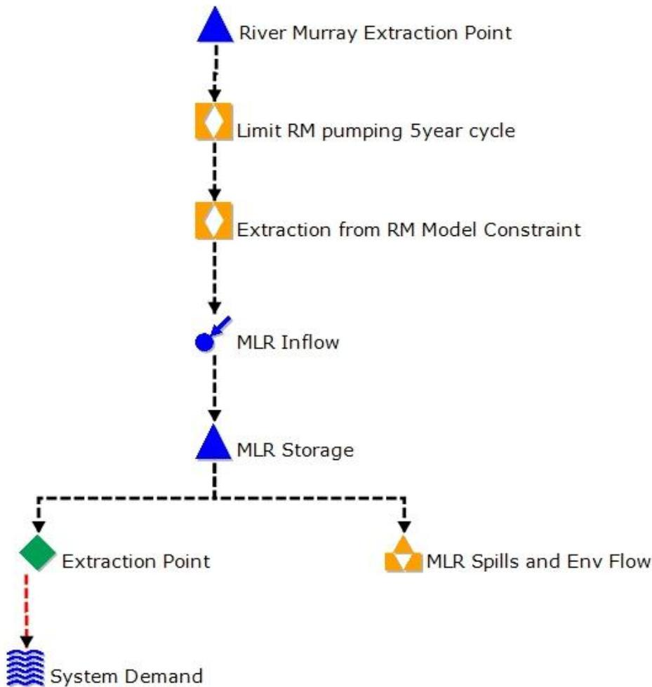
**Figure 15: A schematic diagram illustrating the modelling method adopted for extracting water from the River Murray**
