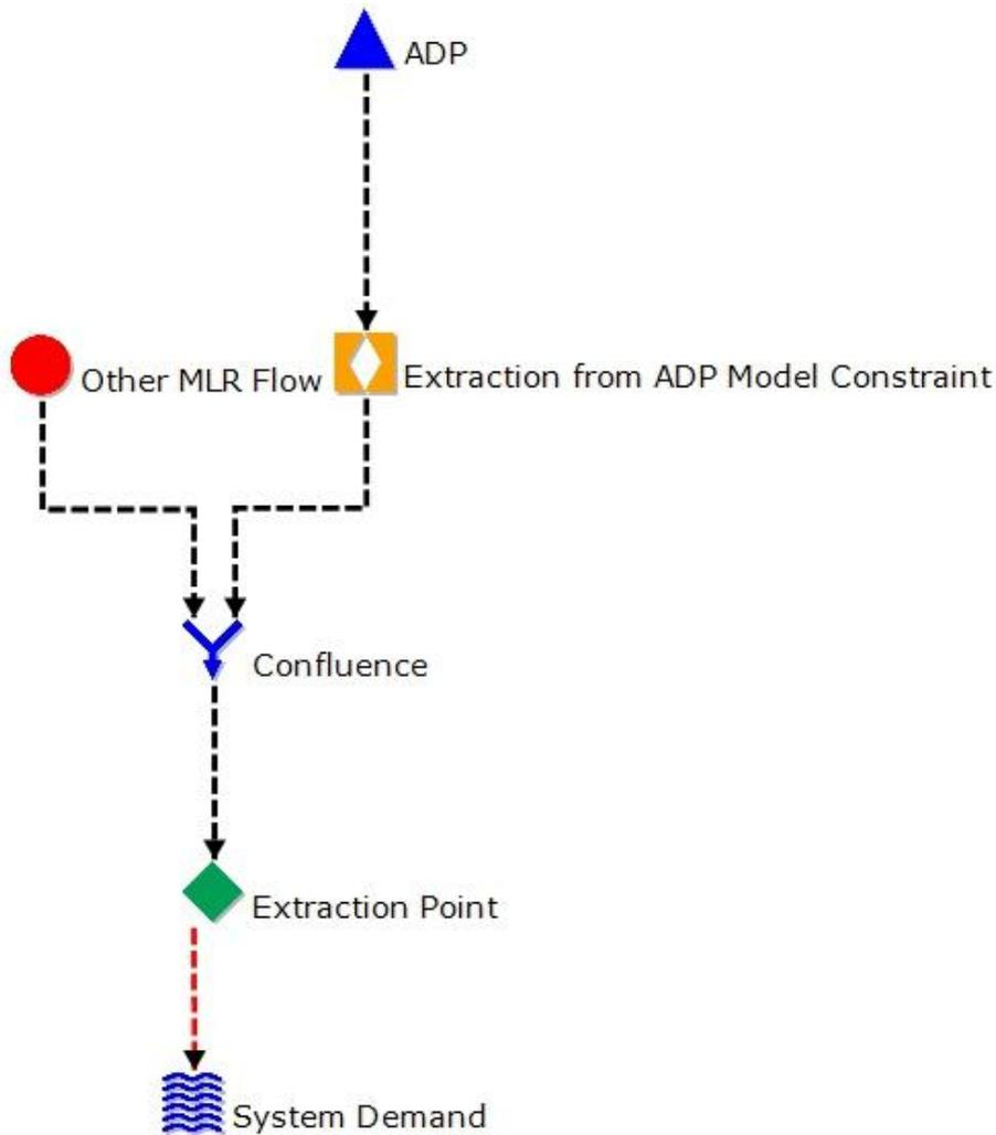
Figure 21: A schematic diagram showing the modelling method adopted for sourcing water from the ADP
