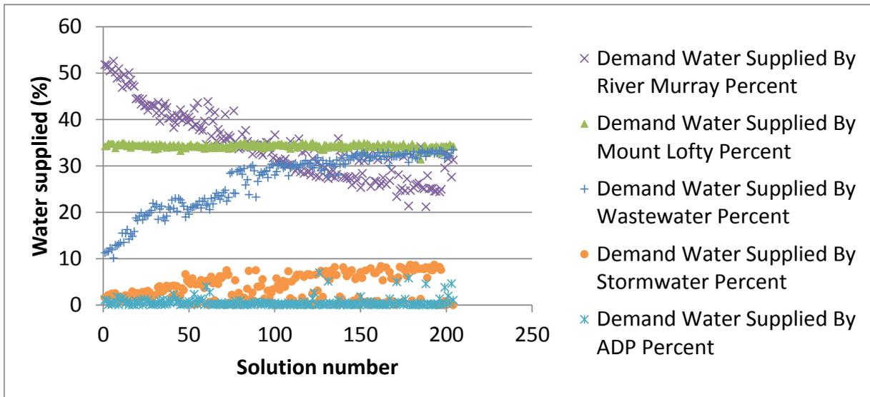
Figure 71: Water supplied by the various sources: Mount Lofty (ML), Murray River (MR), Adelaide Desalination plant (ADP), stormwater (SW) and wastewater (WW) of non-dominated solutions using 2 different seeds (0.123 and 0.147) for the 2050 scenario with Priority Sets #1 and #2
