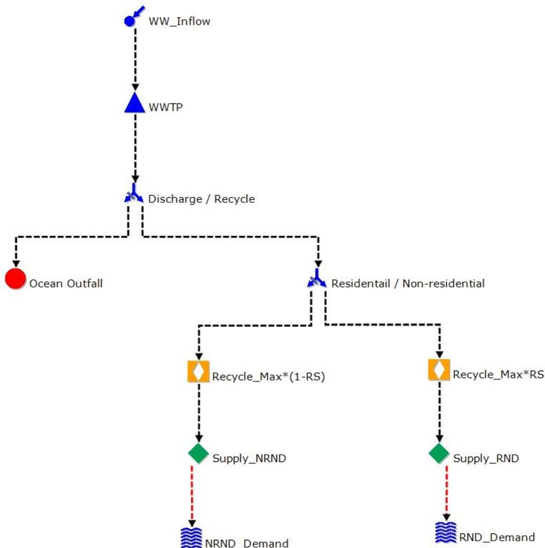
**Figure 23: Schematic diagram illustrating wastewater treatment and reuse modelling method**
