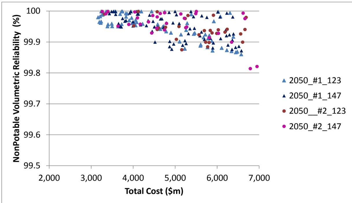
Figure 61: Costs and non-potable volumetric reliability of non-dominated solutions using 2 different seeds (0.123 and 0.147) for the 2050 scenario with Priority Sets #1 and #2
