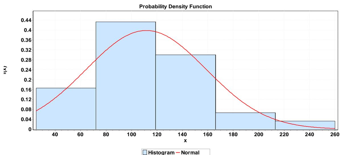
**Figure 37: Connected roof area of households with internally plumbed rainwater tanks (source: Biermann *et al.*, 2012) (Kolmogorov-Smirnov test statistic = 0.182, accepted at 20% significant level; p-value = 0.244)**
