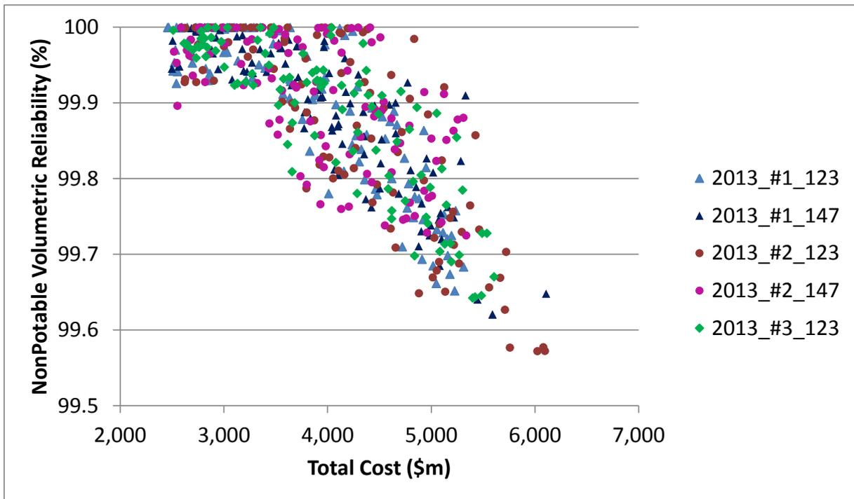
Figure 52: Total costs and volumetric reliability of the solutions found for the 2013 scenario with Priority Sets #1, #2 and #3
