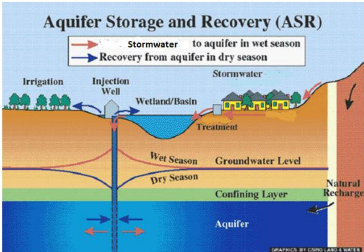
Figure 28: Stormwater harvesting method – Aquifer Storage and Recovery (Image sourced from: CSIRO)
