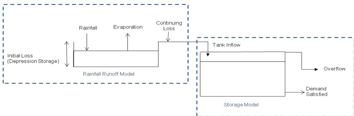
**Figure 35: Schematic representation of the rainwater tank model (source: Neumann 2011, adapted from Mitchell et al., 2008)**
