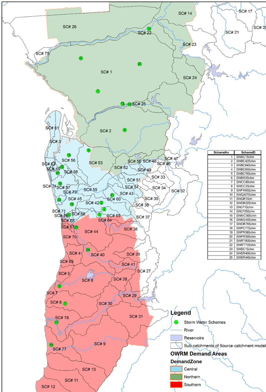
Figure 29: Locations of Lumped stormwater harvesting schemes (note: approximate locations only, i.e. scheme ID is shown at the outlet of the sub-catchment within which the scheme is located)
