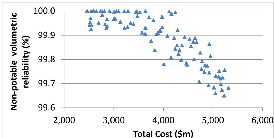
Figure 44: Results of costs and non-potable volumetric reliability for the 2013 scenario with Priority Set #1 and seed 0.123
