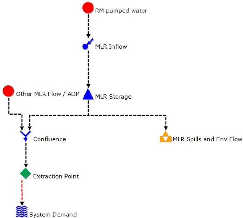
Figure 16: A schematic diagram illustrating sourcing water from a storage in the MLR catchment
