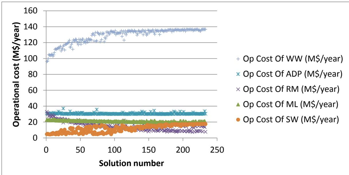
Figure 58: Operational costs of the various sources: Mount Lofty (ML), Murray River (MR), Adelaide Desalination plant (ADP), stormwater (SW) and wastewater (WW) of non-dominated solutions using 2 different seeds (0.123 and 0.147) for the 2013 scenario with Priority Sets #1 and #2
