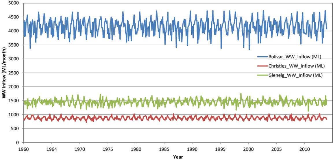
**Figure 27: Modelled monthly wastewater inflow for 2013 scenario by considering the climatic variability during 1960 to 2013**
