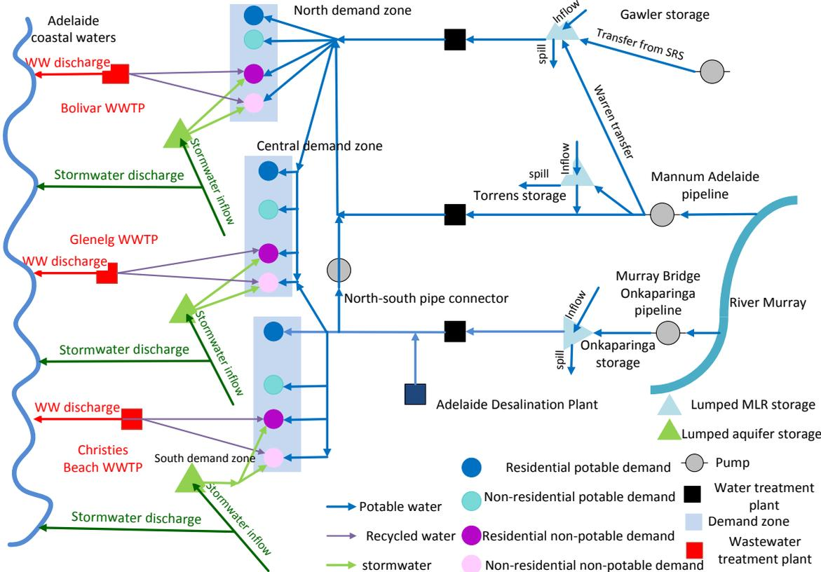
**Figure 14: A schematic diagram showing supply from River Murray, MLR catchments, ADP, wastewater and stormwater sources to residential and non-residential, potable and non-potable demands**
