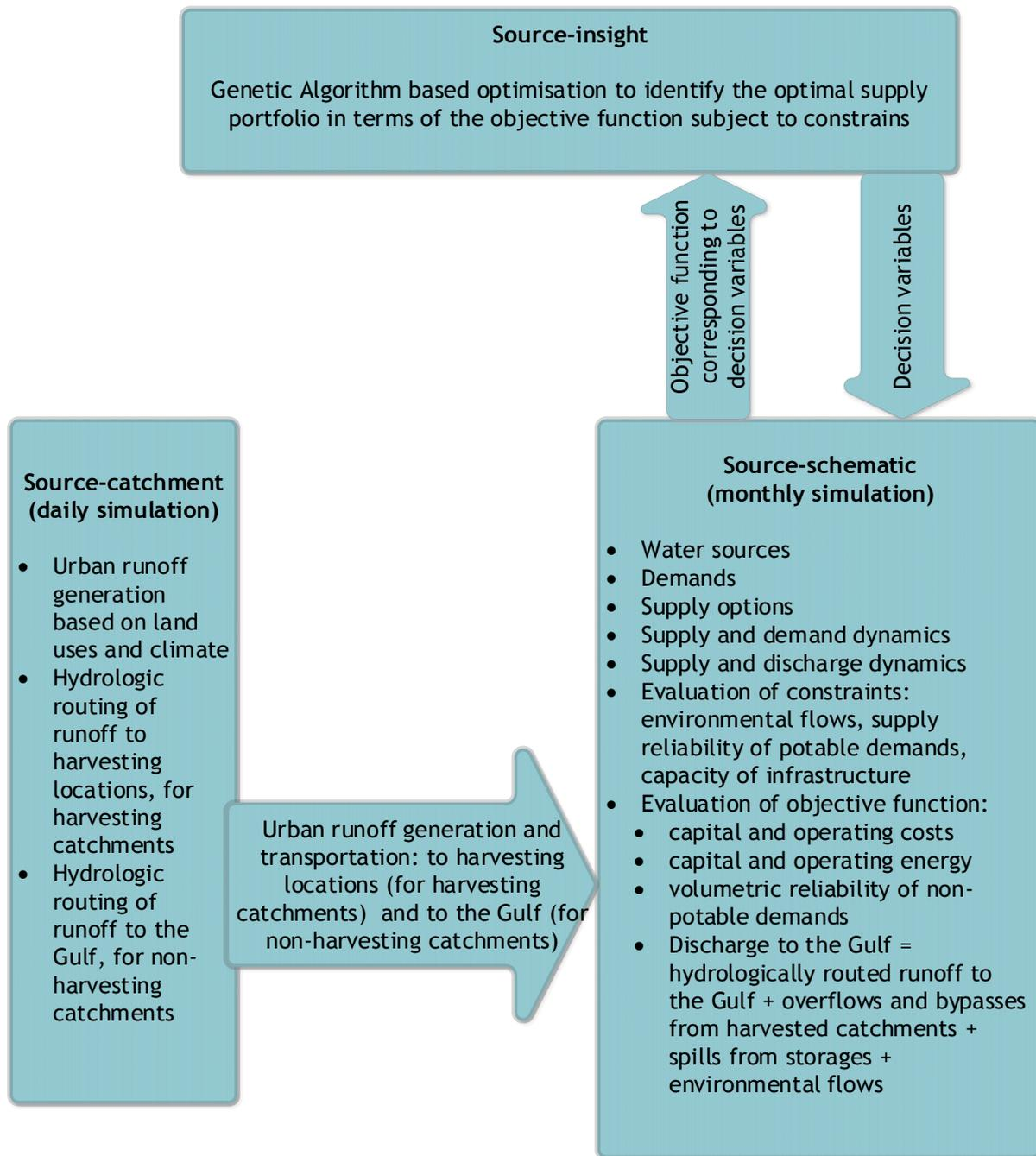
**Figure 13: Interactions between Source modules and how the Source model was used in the IUWM DSF**
