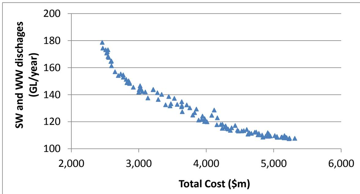
**Figure 45: Results of costs and total stormwater and wastewater discharges for the 2013 scenario with Priority Set #1 and seed 0.123**
