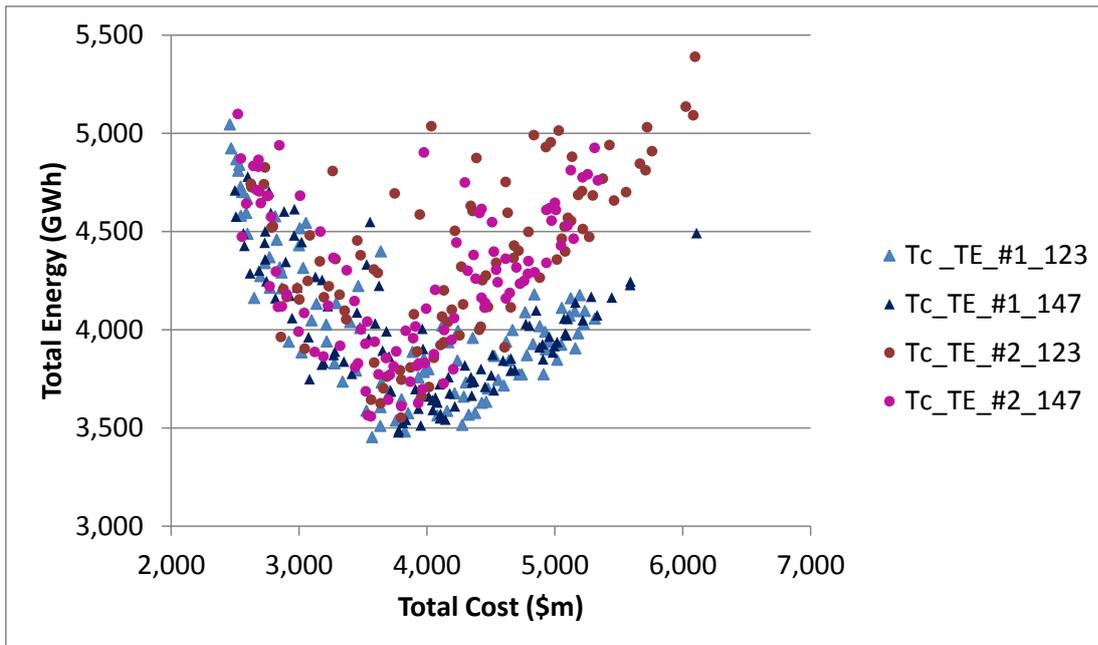
**Figure 46: Results of costs and energies of 2 different seeds (0.123 and 0.147) for the 2013 scenario with Priority Sets #1 and #2, where Tc = total cost, and TE = total energy**
