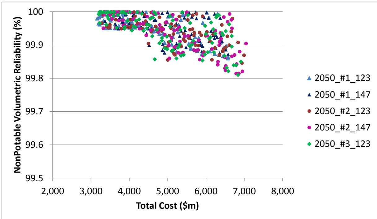
Figure 64: Total costs and volumetric reliability of the solutions found for the 2050 scenario with Priority Sets #1, #2 and #3
