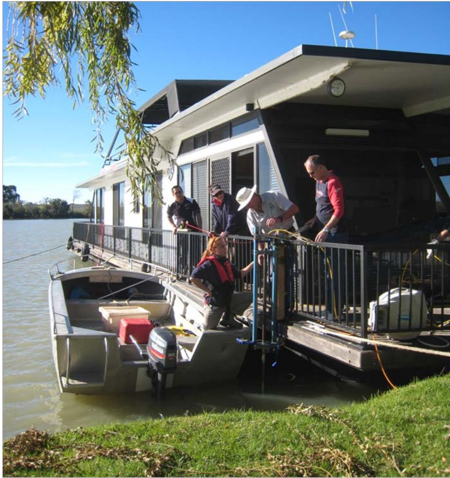
Figure 40: Offshore CPTu setup used in 2013.
