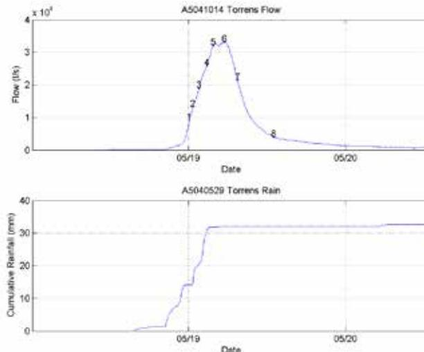
**ApxFigure A-4 Automatic sampler installation (left), and example hydrograph with sample collection times shown (right)**
