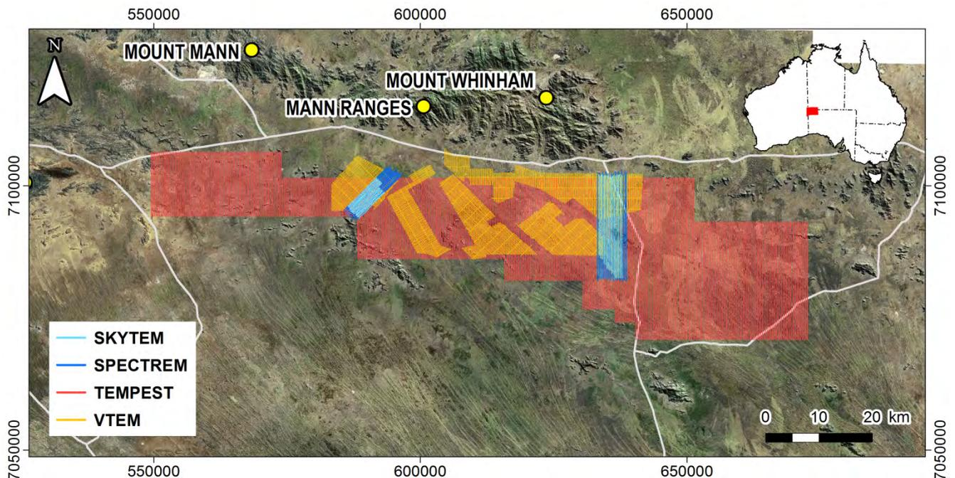
Figure 1. SPECTREM, SkyTEM and historical VTEM and TEMPEST flight paths overlaid on an orthophotograph of the area.
