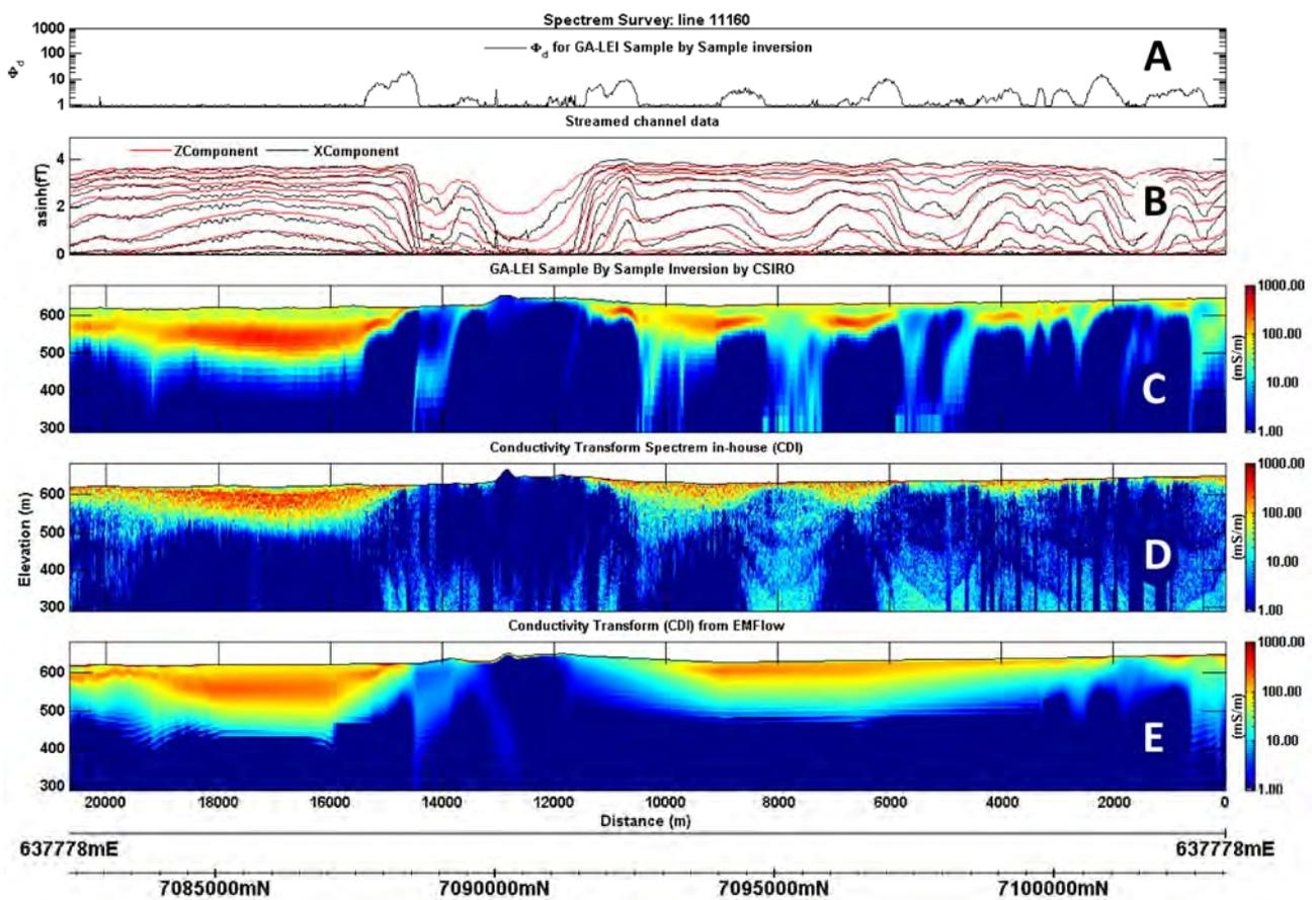
Figure 8. Profiles of line 11160 showing  $\phi_d$  panel A, 10 channels of Z- and X-component measured data panel B, two CDI conductivity–depth sections provided by the Spectrem Air Ltd (panels D and E respectively), and a GA-LEI inverted section (panel C). To allow meaningful comparison, the three conductivity–depth sections are displayed with the same colour scale.
