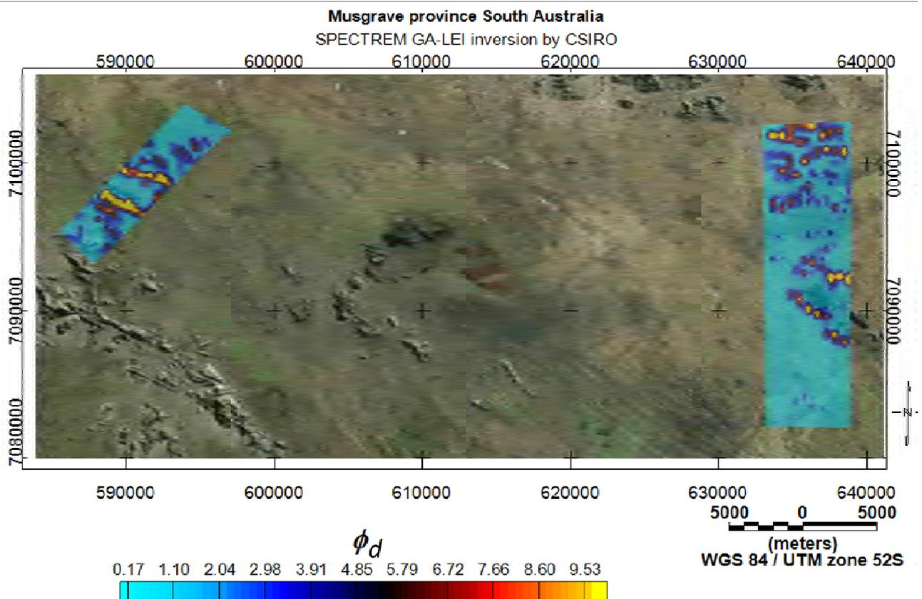
Figure 7. Spatial distribution of parameter  $\phi_d$  draped over an SRTM image. Larger misfit are seen around areas of outcrop and on the margins of depressions filled with sediment.
