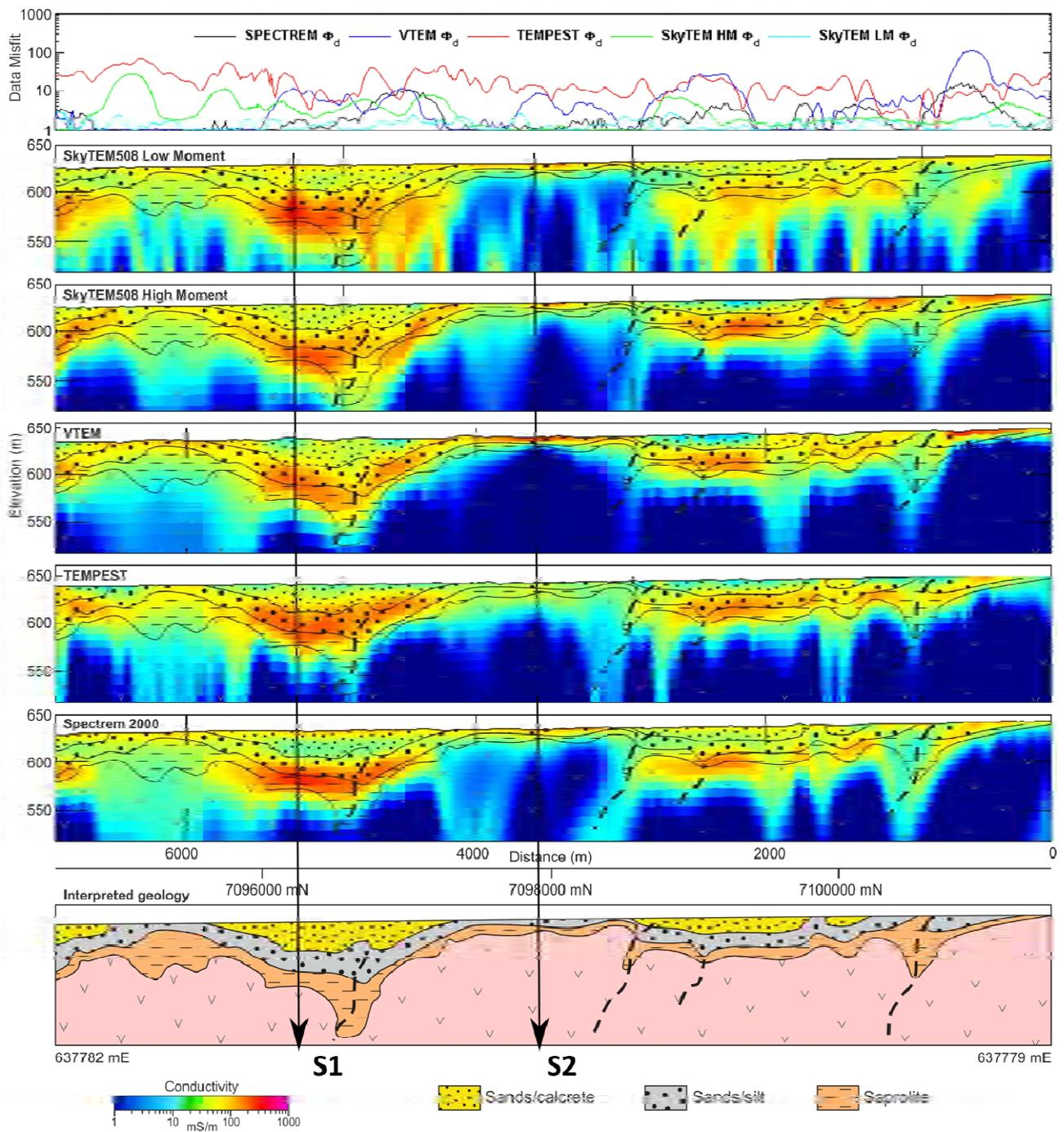
Figure 16. Comparison of 30-layer inversions of four coincident north–south lines flown in 1998, 2011 and 2012 using Tempest, VTEM, SkyTEM<sup>508</sup> and SPECTREM<sub>2000</sub>AEM systems. Interpreted geology (from limited off-section drilling) is superimposed.
