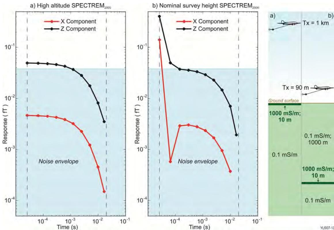
Figure 6. Modelled X and Z component responses, in panel a) from a transmitter dipole at 1000 m altitude over a 10-m-thick of 1000 mS/m conductivity conductor at the surface. Panel b) shows responses from dipole at a nominal altitude of 90; with the same 1000 mS/m conductor at a depth of 1000 m below a resistive (1 mS/m) host.
