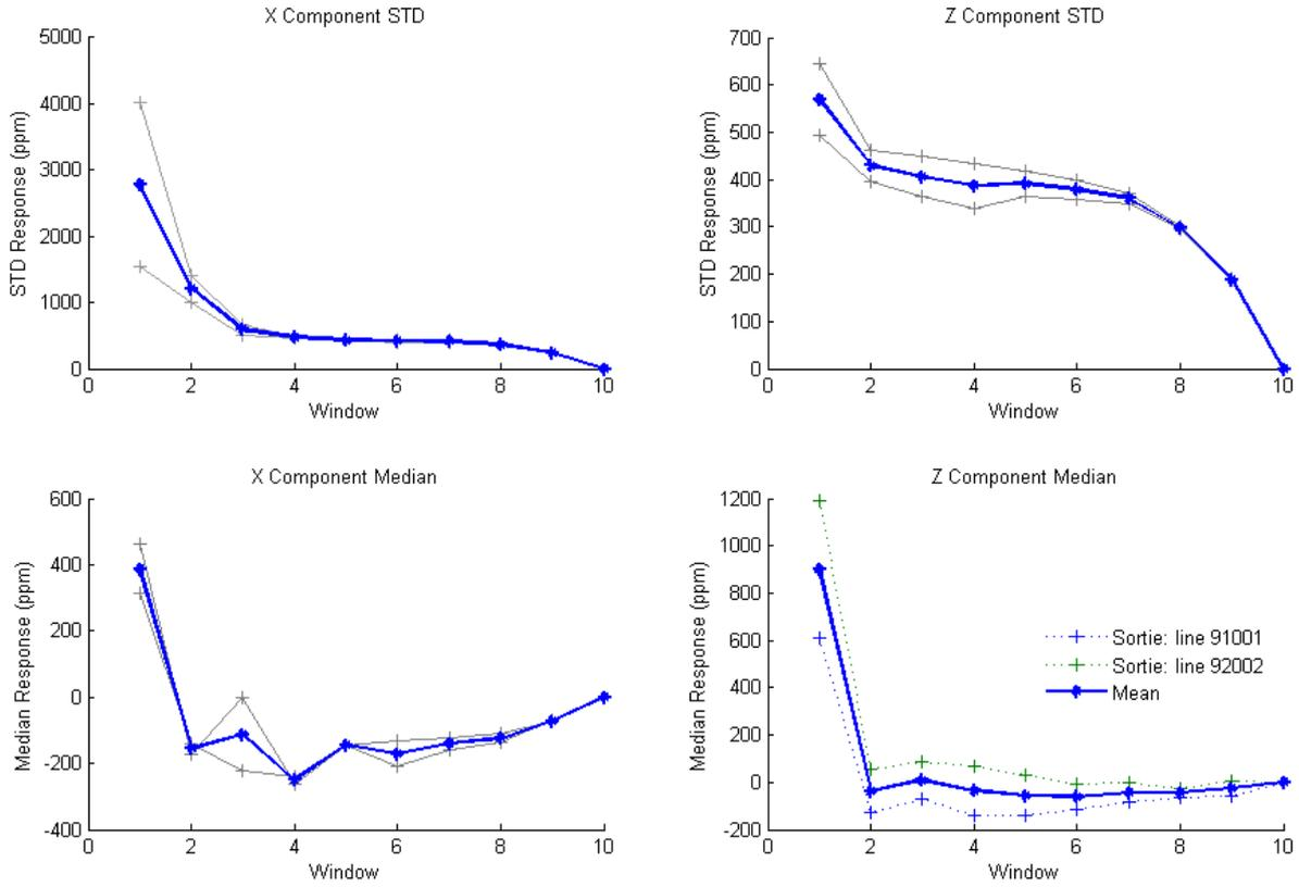
Figure A1. Noise levels for each window of both X and Z components estimated during high-altitude flight, assuming the signal is recorded in the absence of ground response.
