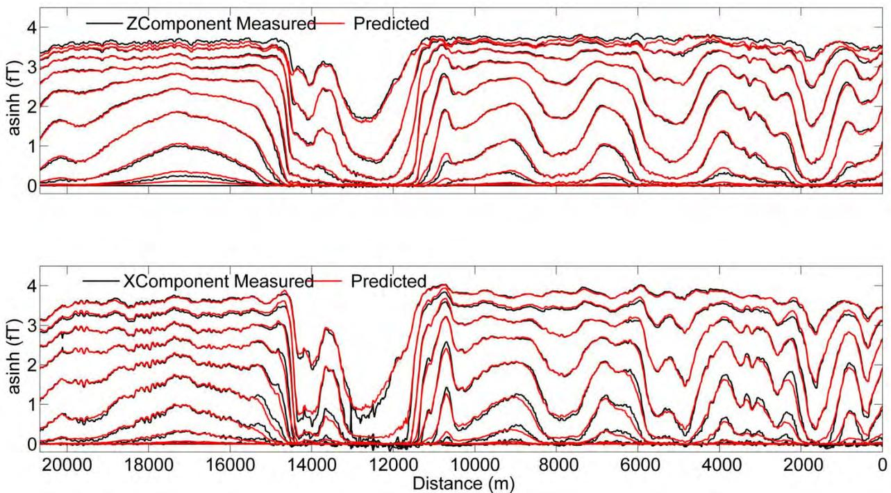
**Figure 10 Profile of line 11160 showing 10 channels of X and Z-component measured data (black) and forward-modelled response from best-fit model (red).**
