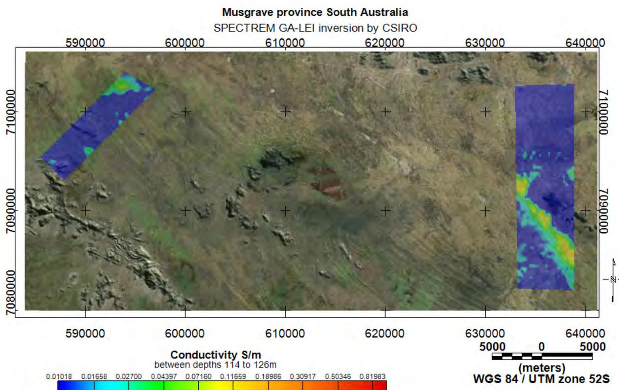
Figure 13. Conductivity–depth interval from 114 to 126 m below the surface.
