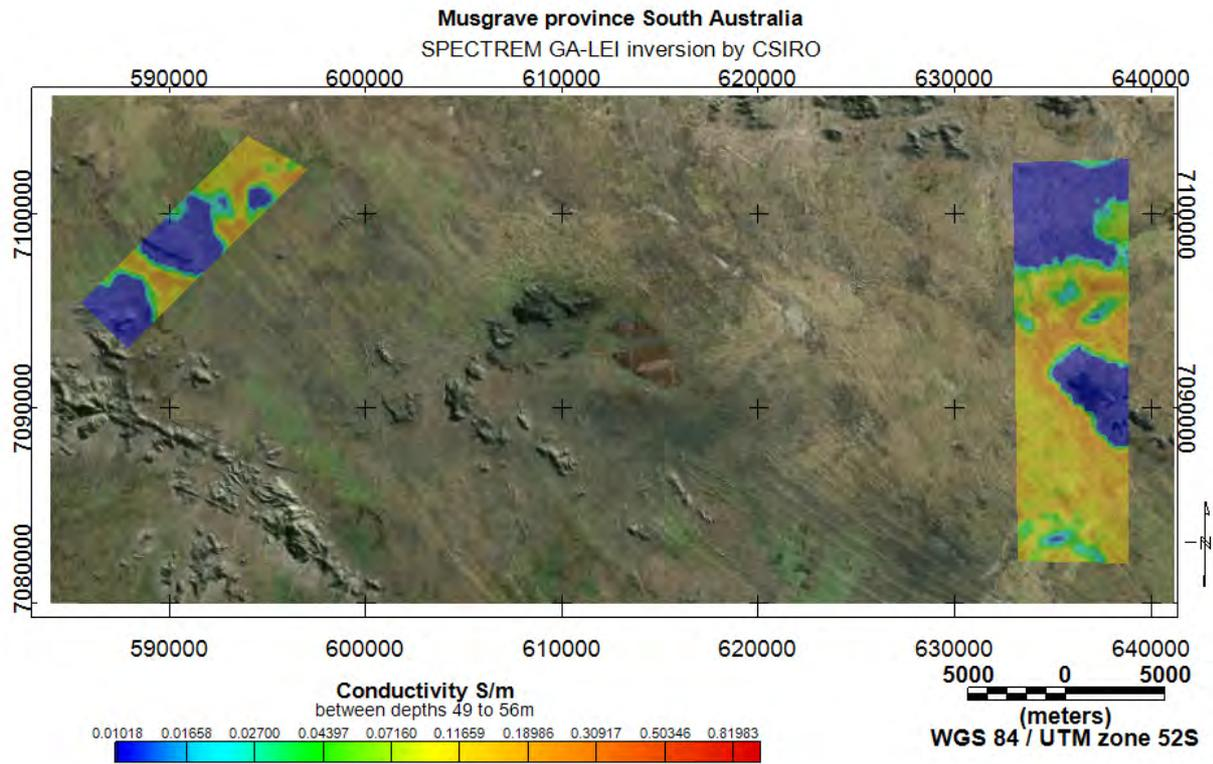
Figure 14. Conductivity–depth map from 49 to 56 m below the surface.
