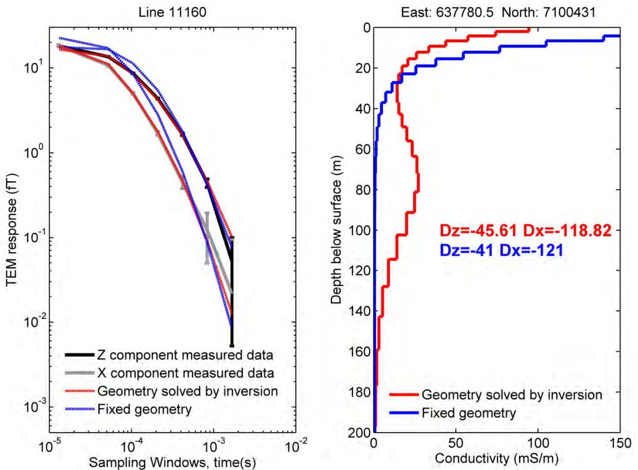
Figure 5. Inversion results for one sounding on line 11160. The grey and black decays on the left hand panel are X and Z component total field data plotted with each time gate's associated error-bar. Also shown are responses of the best fitting 30 layer forward models resulting from inversions where the geometry remained fixed (blue), and was included to be solved for in the inversion (red). The right hand panel shows the corresponding best fit conductivity-depth models in the same colours.
