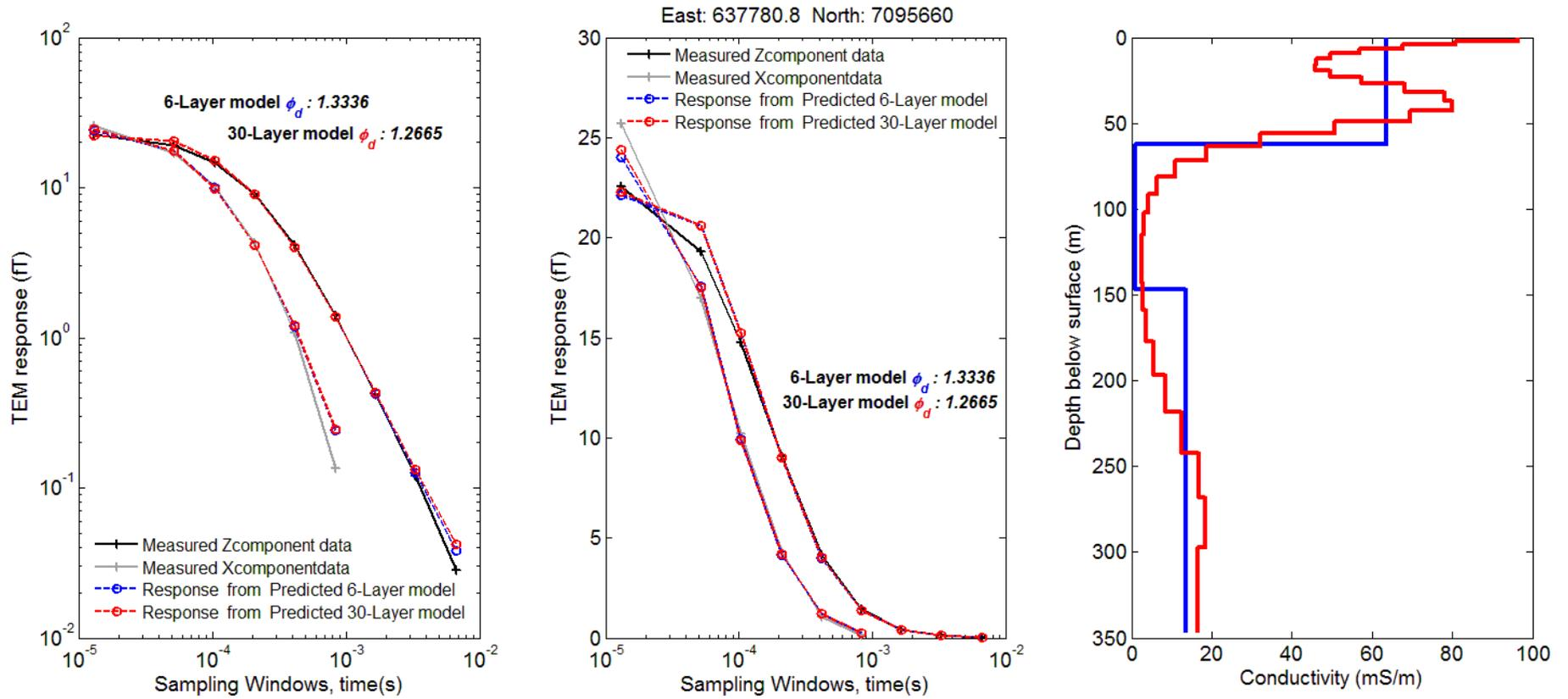
Figure 11. Measured data and predicted responses from a 6-layer and 30-layer inversion, for one sounding. The inversion fails to fit the observed data at early and late times. Left panel plot is on a log-log scale; middle panel log-linear and right panel shows the two proposed conductivity-depth models.
