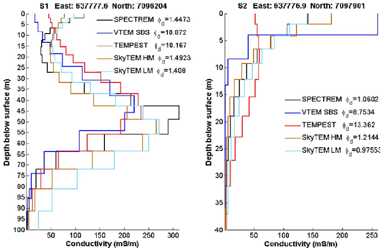
Figure 17. Comparisons of individual soundings for SPECTREM, VTEM, TEMPEST and SkyTEM data at two locations along coincident lines after inversion with the 30-layer starting model for the GA-LEI inversion. The two soundings show recovered models from all system over conductive and resistive area.
