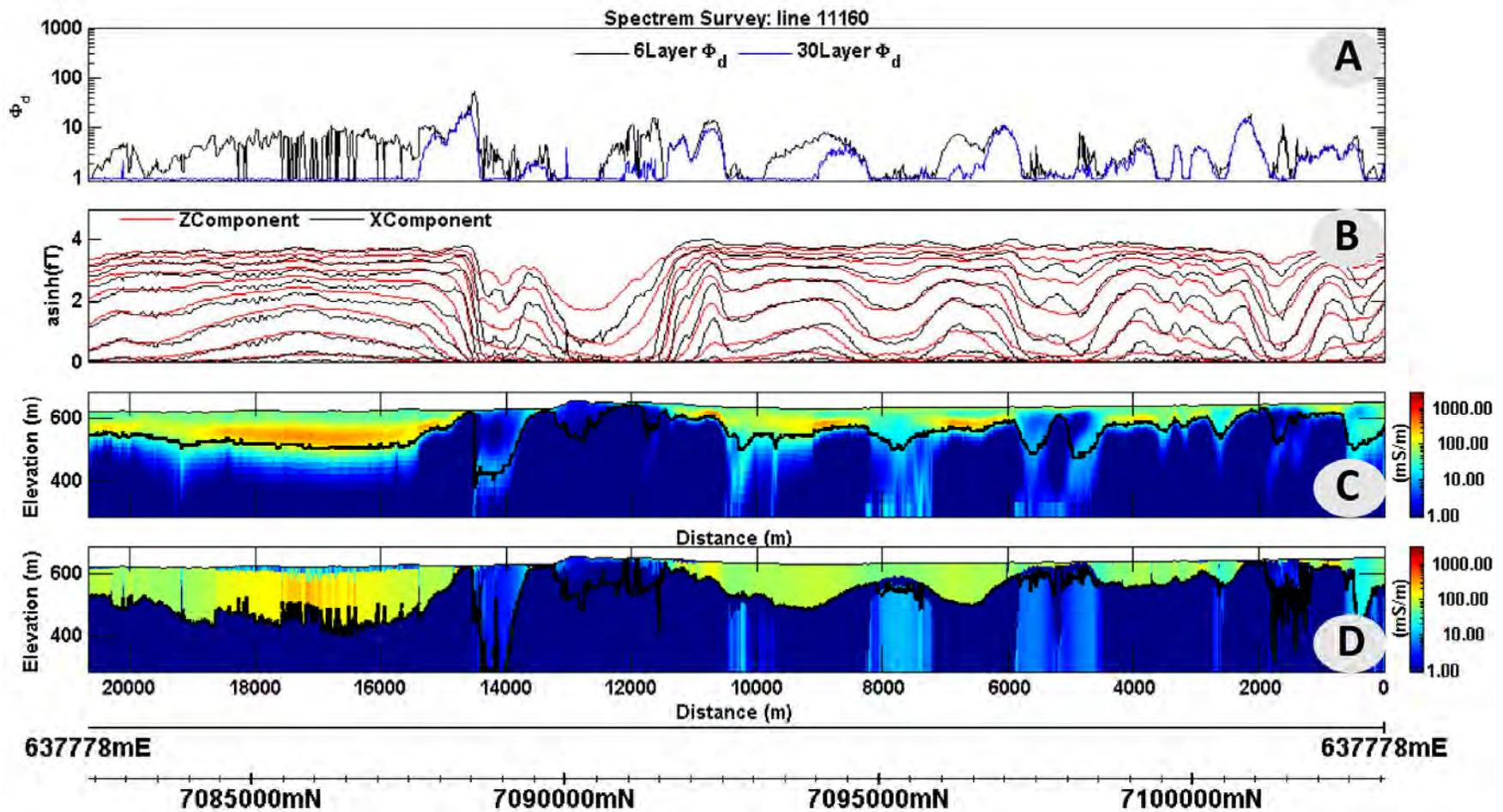
Figure 12. Line 11160 of SPECTREM data from the Musgrave province survey. Panel A shows how the data can be represented by a 1D model (parameter  $\phi_d$ ). Panel B shows processed channel X- and Z-component data. Panel C shows a 30-layer inversion with fixed layer thicknesses. Panel D shows a 6-layer inversion where both conductivities and layer thicknesses are solved by inversion.
