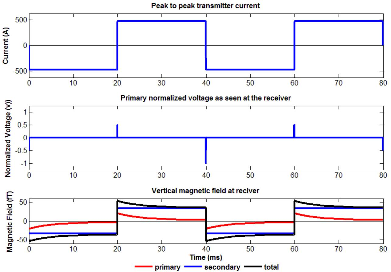
Figure A2. SPECTREM waveform showing a) transmitter current waveform, b) voltages at the receiver for the vertical Z component and c) vertical Z component of the magnetic B-field
