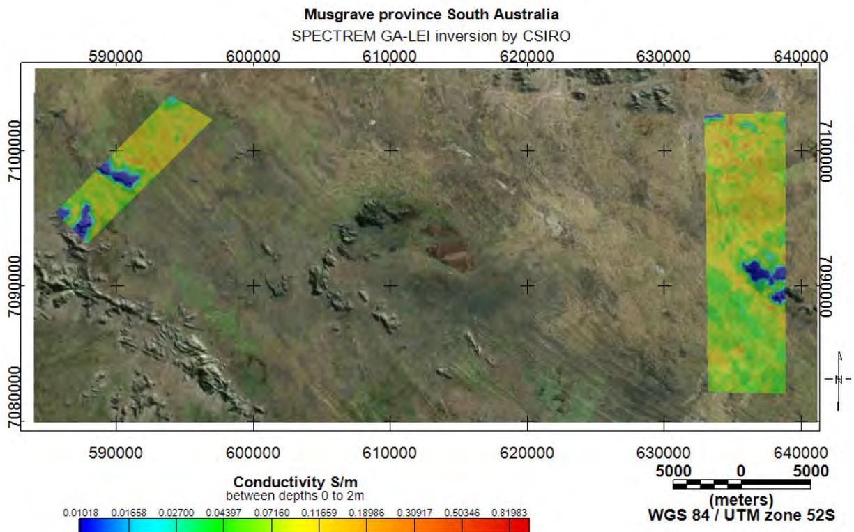
Figure 15. Conductivity–depth range, from 0 to 2 m below the surface.
