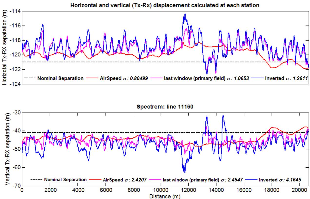
Figure 4. Horizontal (top panel) and vertical (lower panel) transmitter–receiver (Tx–Rx) separations estimated at each fiducial over a 20 km line. Separations and their respective standard deviations were calculated by airspeed (red), last window (magenta), inversion (blue) against the nominal separation (black dashed line).
