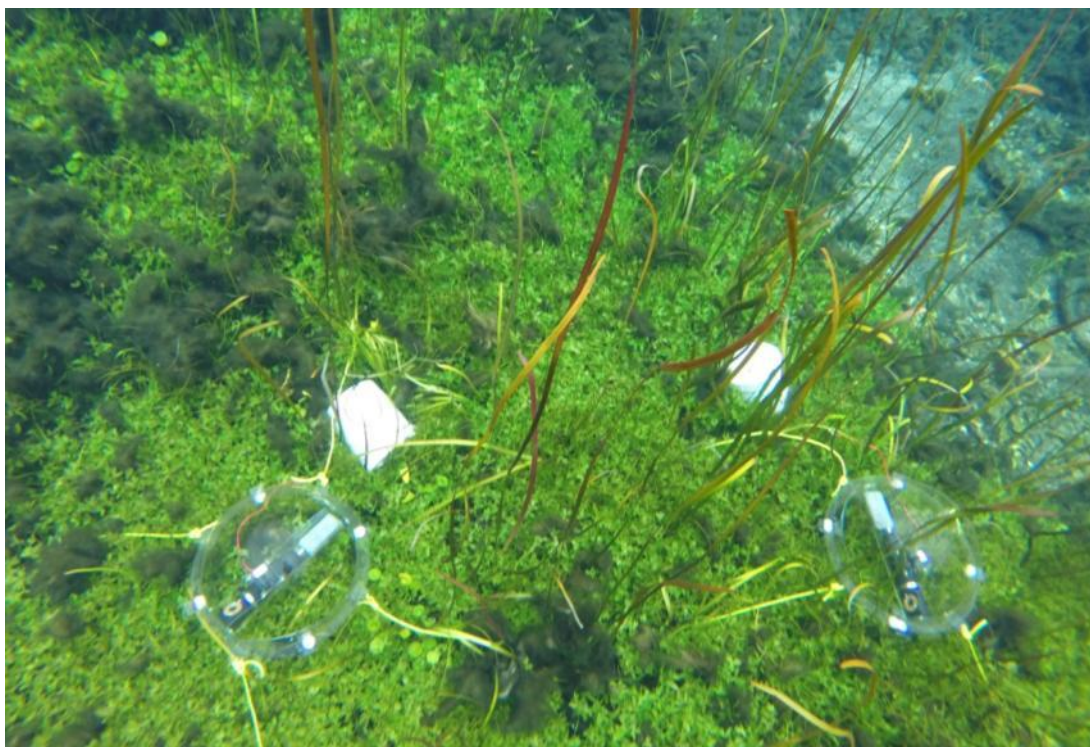
Figure 7. Submerged domes deployment in Ewens Ponds for the photosynthetic activity assessment.
