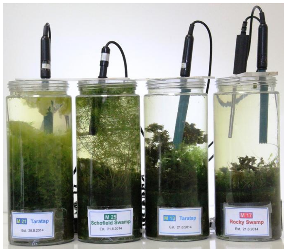
Figure 9. Variation in mesocosm plant composition, and probes for continuous monitoring of pH, Eh, EC and temperature.
