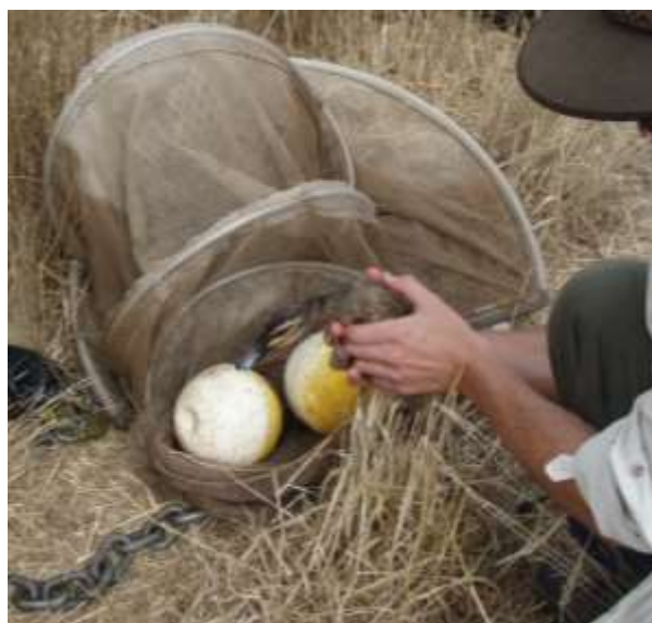
Figure 20. Buoys in cod-end of net to protect air-breathing fauna.
