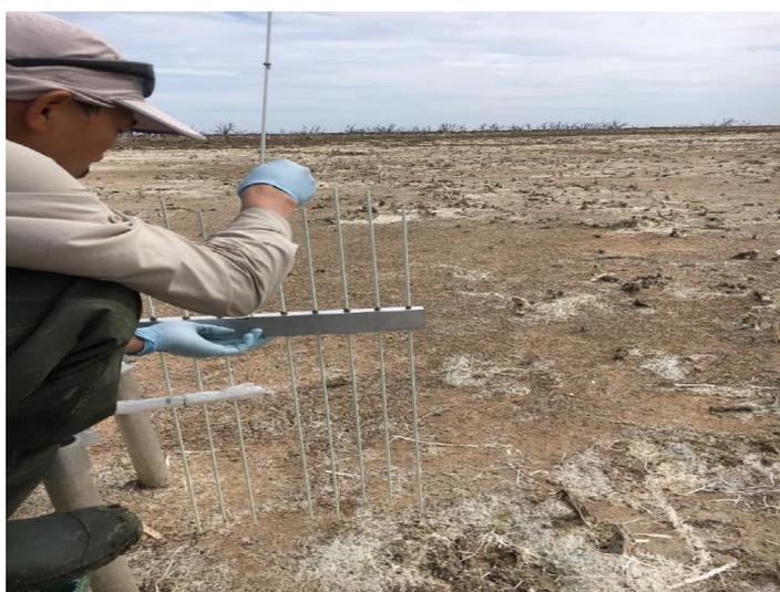
Figure 12. Photo of a sediment elevation table in the trial pond.
