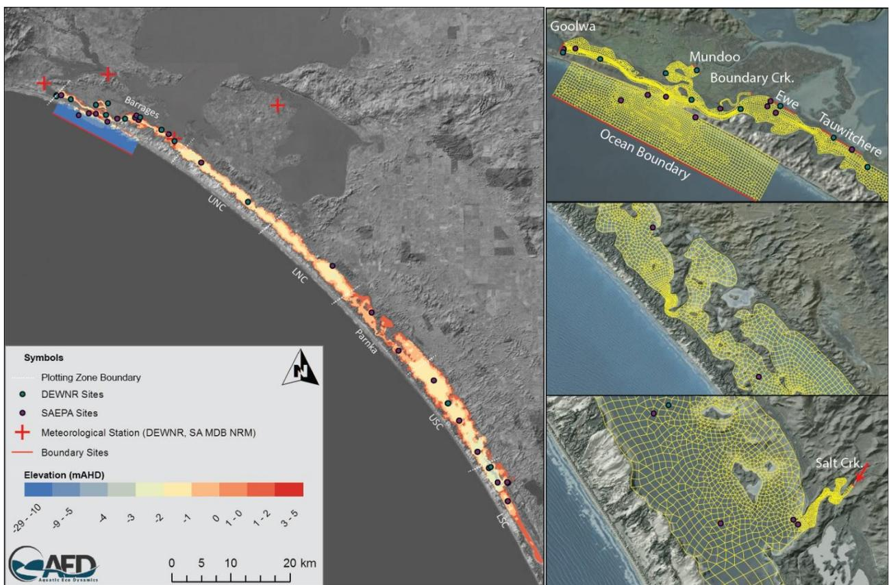
Figure 1. Outline of the simulated model domain, indicating the model mesh, analysis regions, and monitoring sites.
