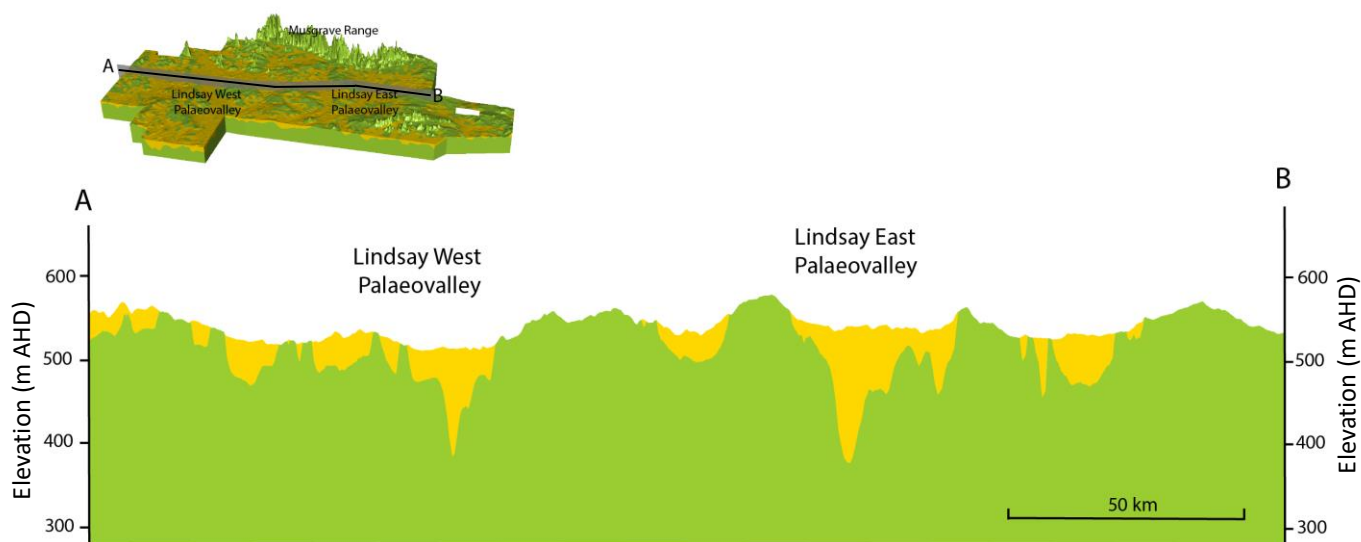
Figure 4-24. West-east geological cross-section through the Lindsay West and Lindsay East palaeovalley systems. The orientation of the cross-section is shown in the three-dimensional geological model above the section.
