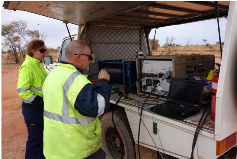
Figure 30. Winch and Borehole nuclear magnetic resonance controller in field data acquisition configuration.
