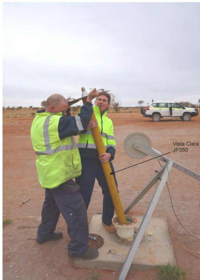
Figure 29. Setting up of the Vista Clara Borehole nuclear magnetic resonance logging tool over DH1a.
