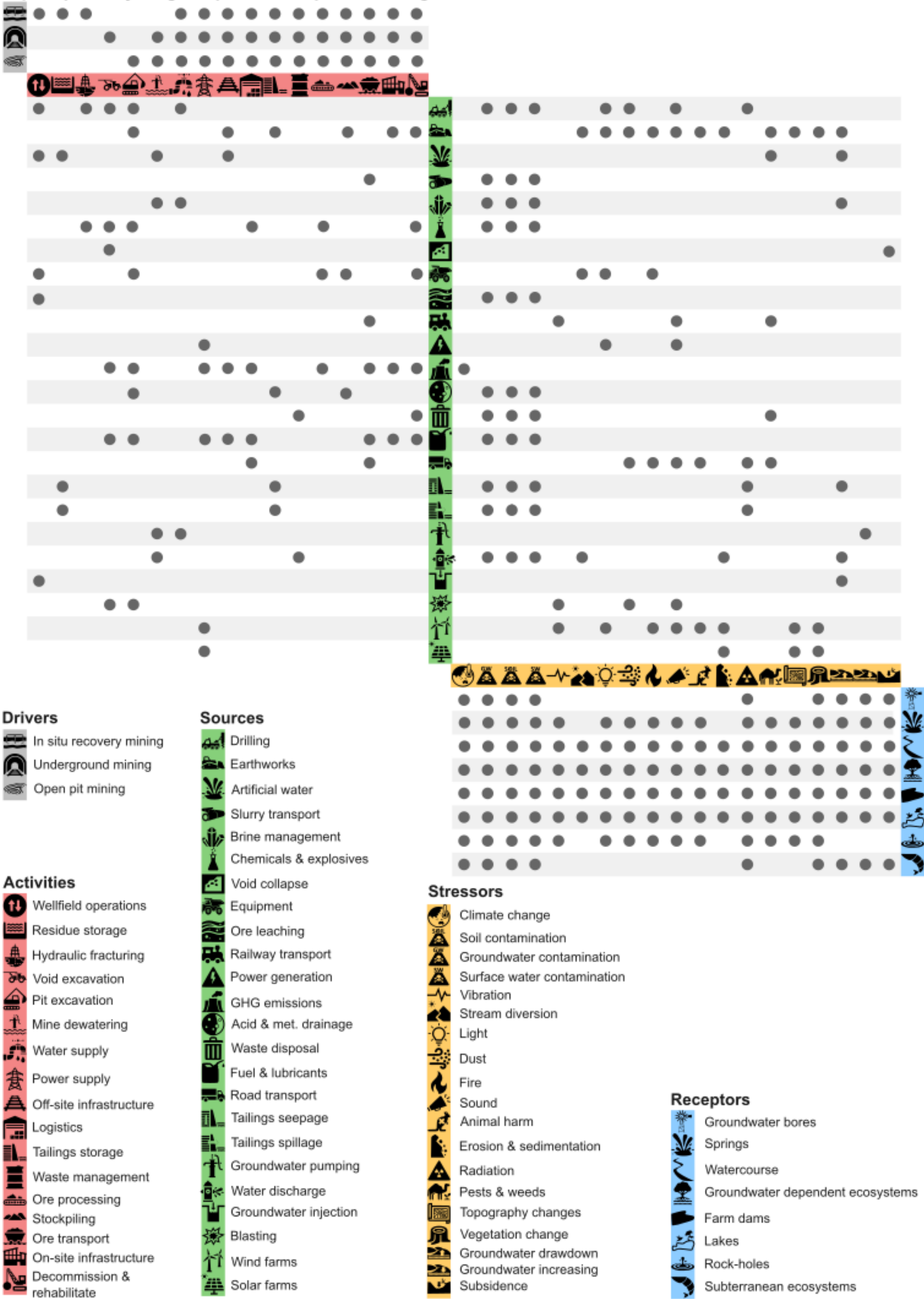
Figure 5 Impact pathway diagram in matrix form for the production phase of open-pit, underground and in situ recovery mining (figure designed to be printed on A3).
